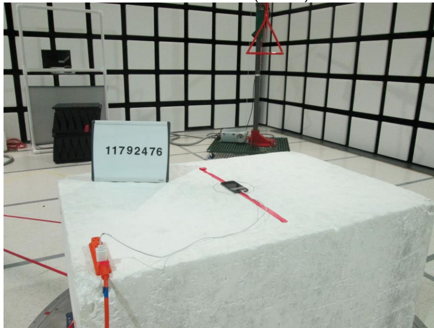
RADIATED EMISSIONS ABOVE 30 MHz (FRONT)
