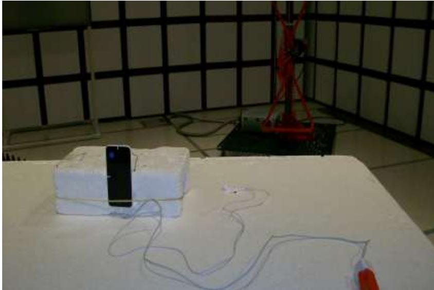
**POWERLINE CONDUCTED EMISSIONS MEASUREMENT SETUP**
