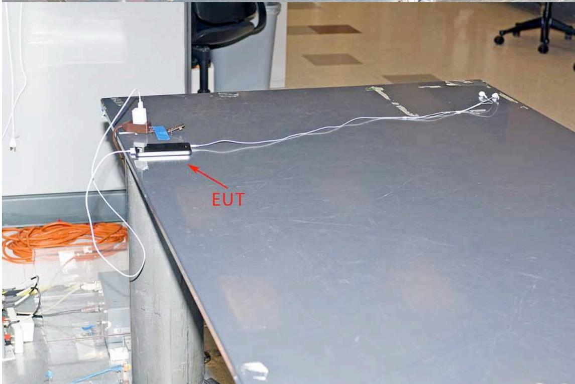
2.14 Radiated Emissions Test Setup Photos
