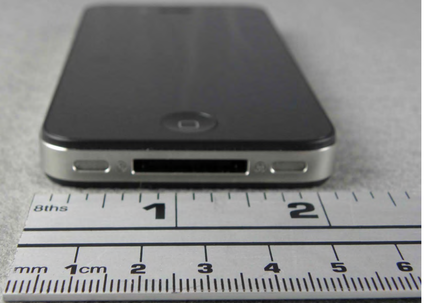
EXTERIOR PHOTO 6 BOTTOM END SPEAKER, MIC, & 30 PIN DOCKING CONNECTOR
