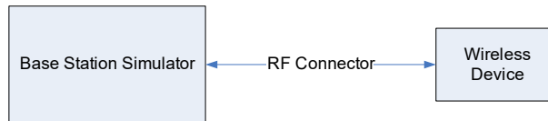
Figure 8-1 Power Measurement Setup
