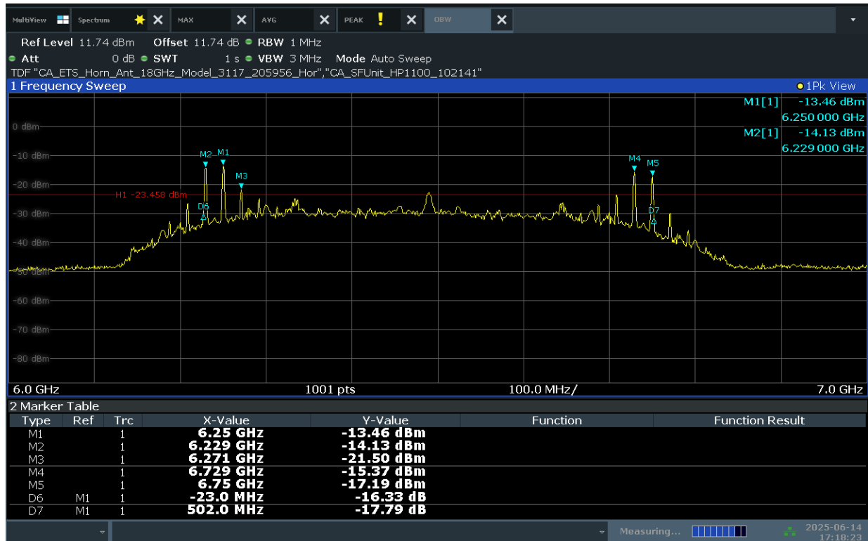
Plot 7-1. 10dBc Bandwidth (Ch. 5, Config 9/Payload 65B)
