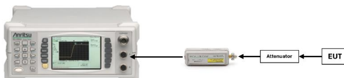
Figure 7-2. Test Instrument & Measurement Setup for Peak and Average Power Measurement
