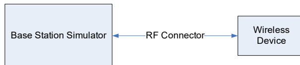
Figure 8-1 Power Measurement Setup
