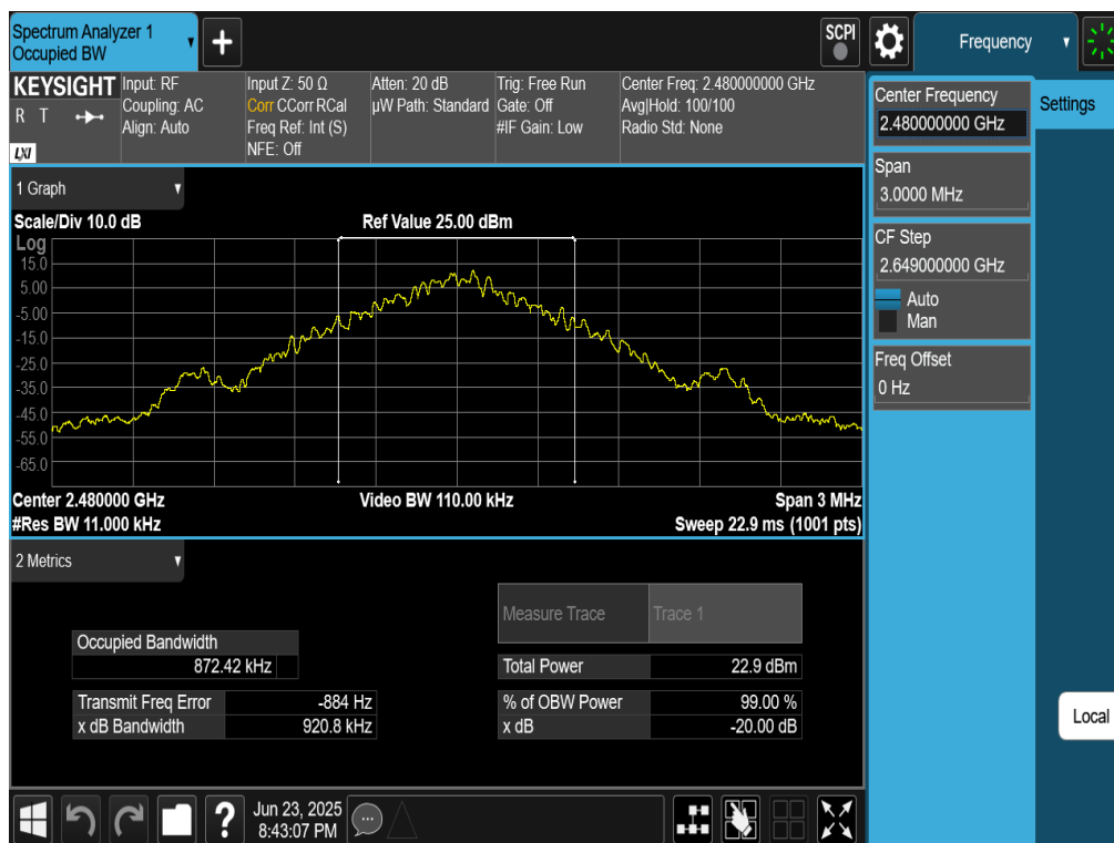
Plot 7-3. 20dB BW and 99% OBW Plot (Bluetooth, GFSK, ePA – Ch. 78)
