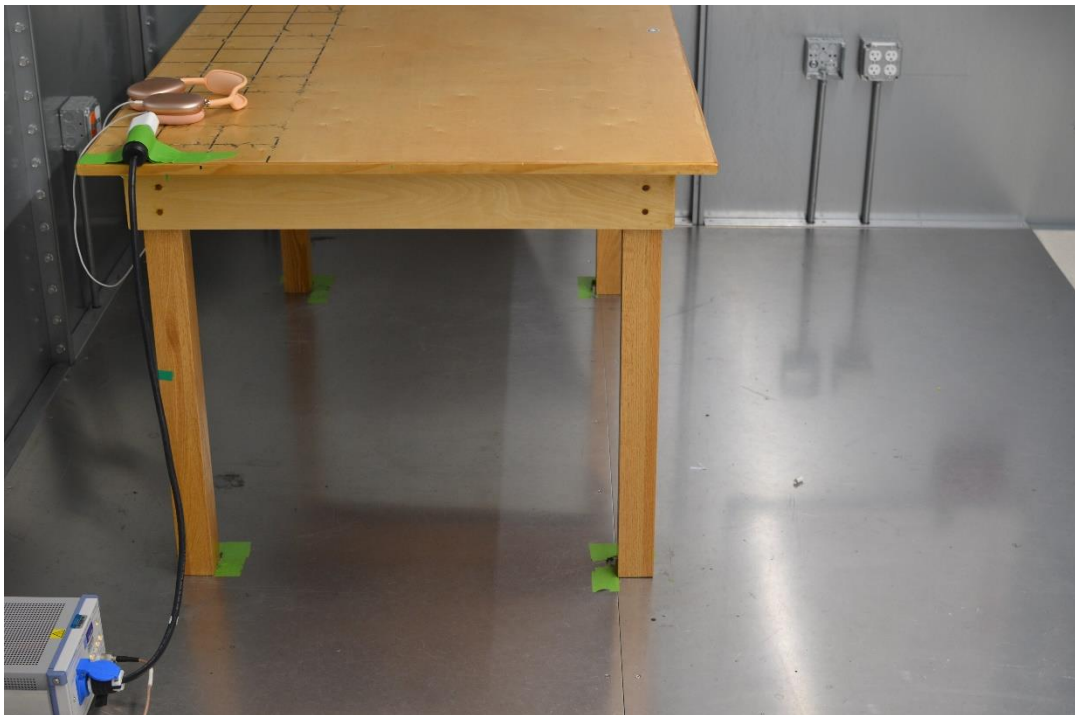
Figure 2: AC Line Conducted Emissions (Side View)
