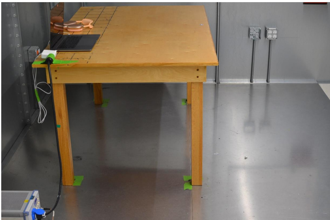
Figure 4: AC Line Conducted Emissions (Side View)
