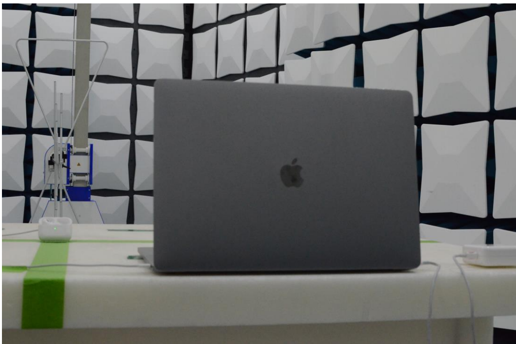
Figure 22: 30MHz-1GHz Test Setup (Rear View)
