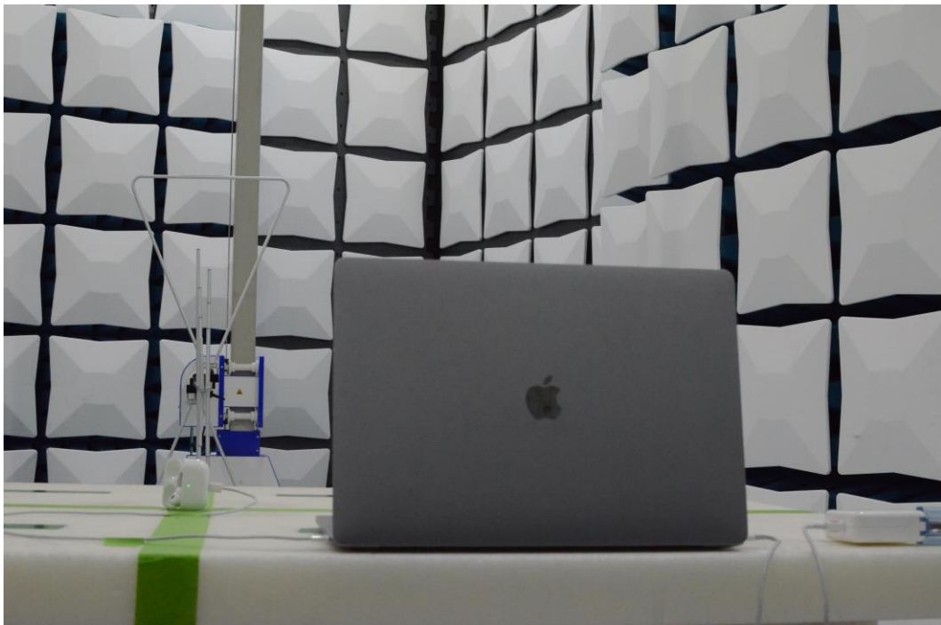
Figure 20: 30MHz-1GHz Test Setup (Rear View)
