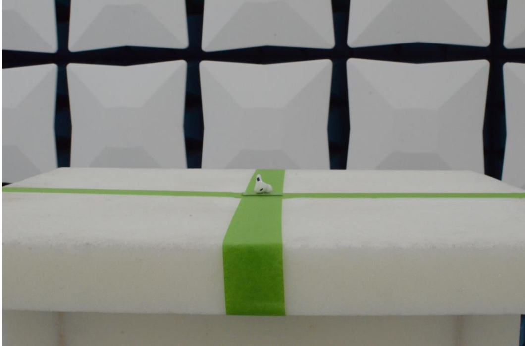
Figure 5: 1-18GHz Test Setup (Front View)
