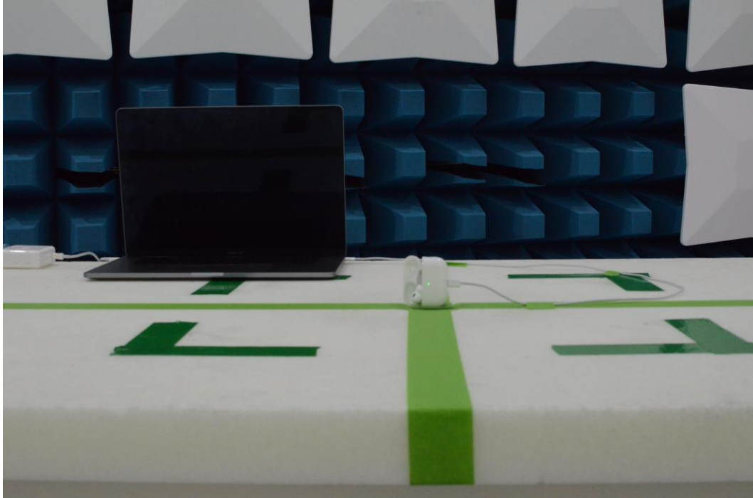
Figure 19: 30MHz-1GHz Test Setup (Front View)
