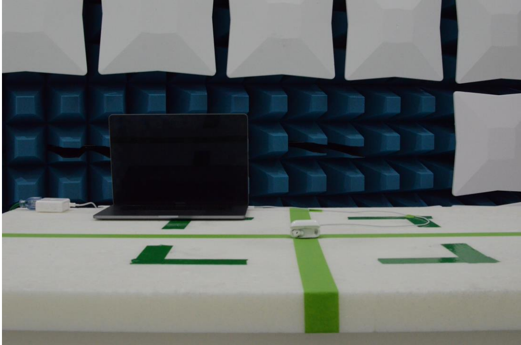
Figure 17: 30MHz-1GHz Test Setup (Front View)
