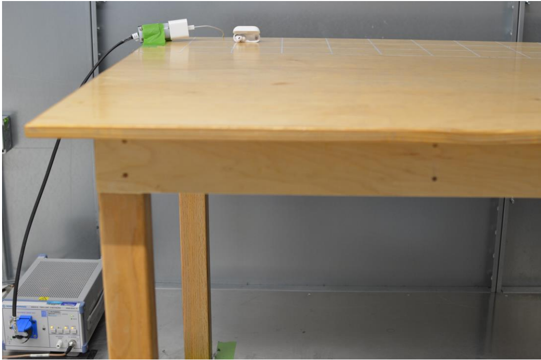
Figure 1: AC Line Conducted Emissions (Front View)
