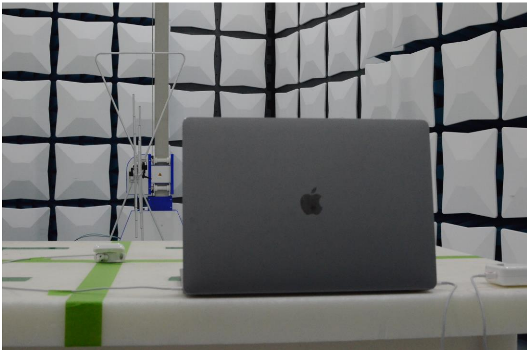
Figure 18: 30MHz-1GHz Test Setup (Rear View)
