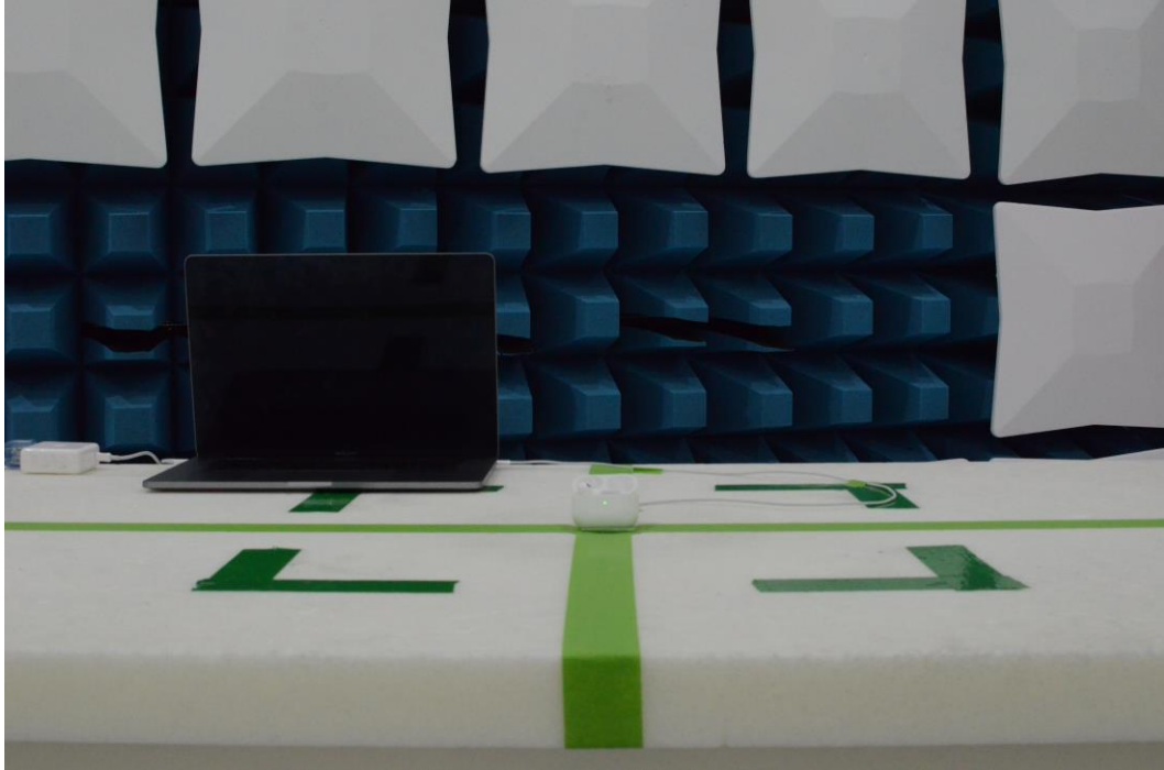
Figure 21: 30MHz-1GHz Test Setup (Front View)
