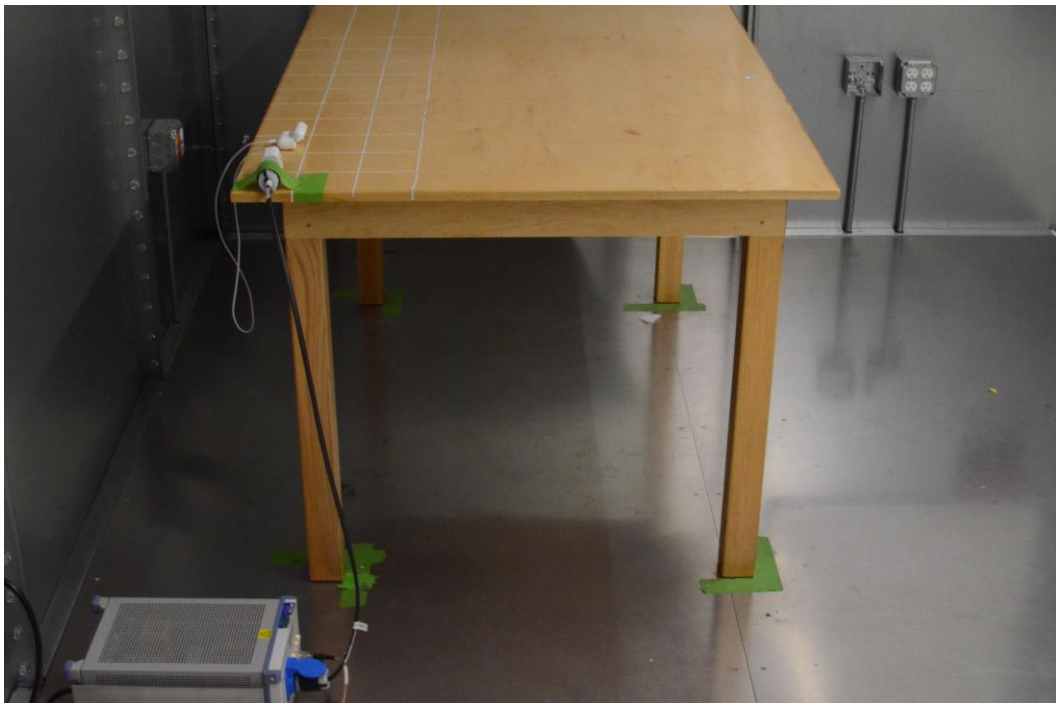
Figure 2: AC Line Conducted Emissions (Side View)
