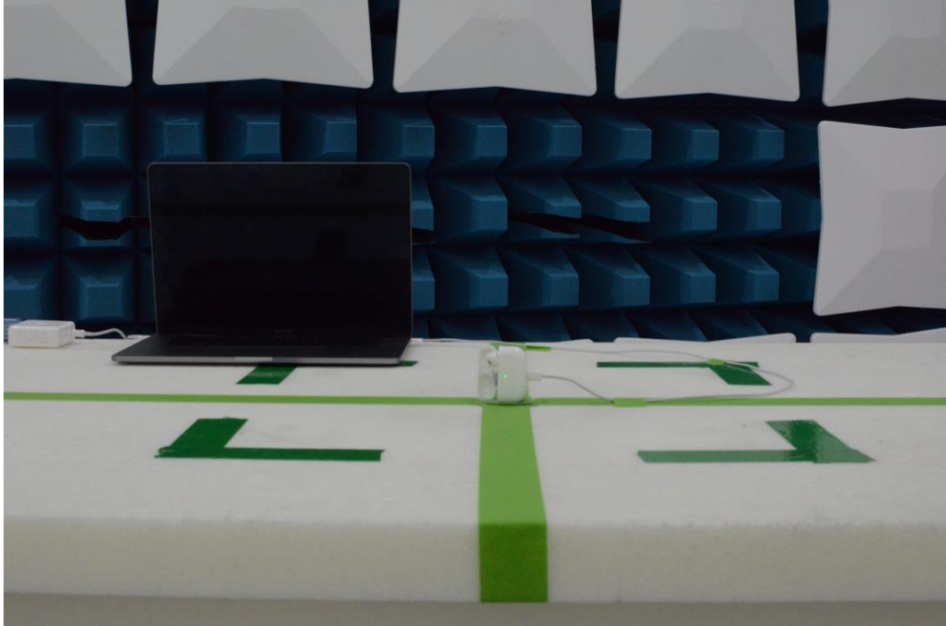
Figure 21: 30MHz-1GHz Test Setup (Front View)
