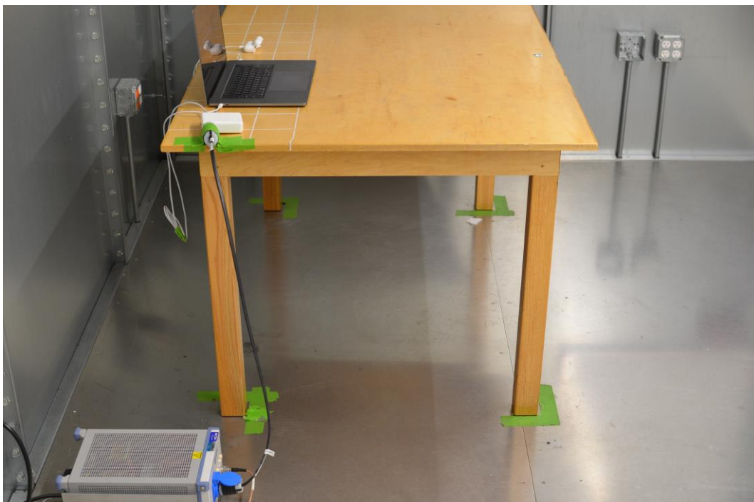
Figure 4: AC Line Conducted Emissions (Side View)
