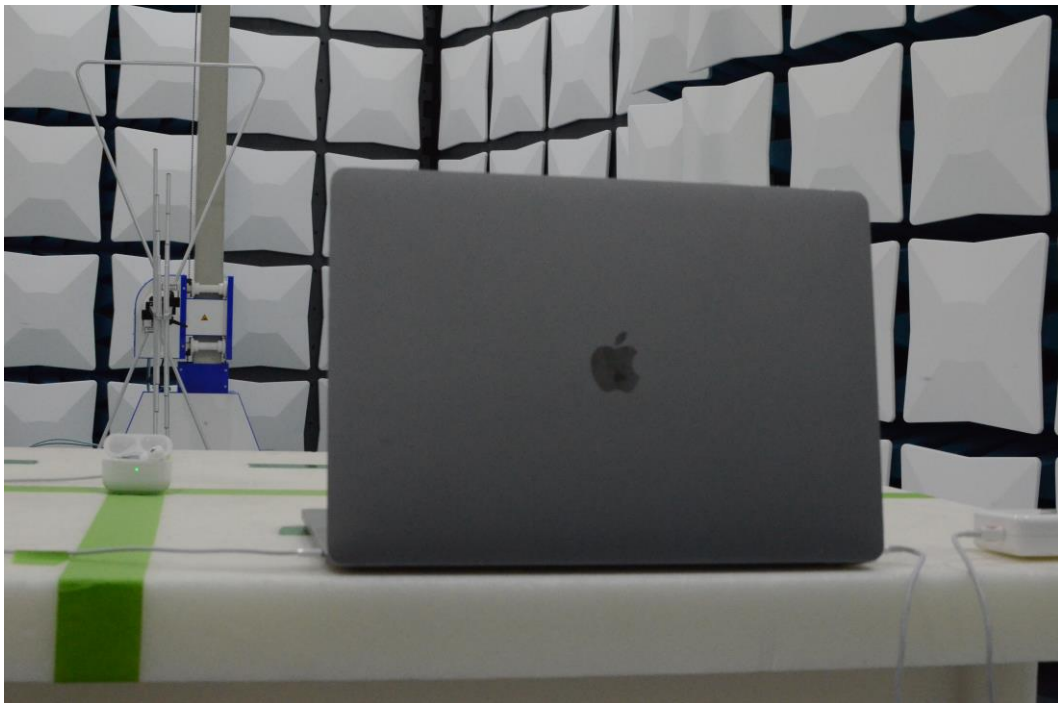
Figure 20: 30MHz-1GHz Test Setup (Rear View)
