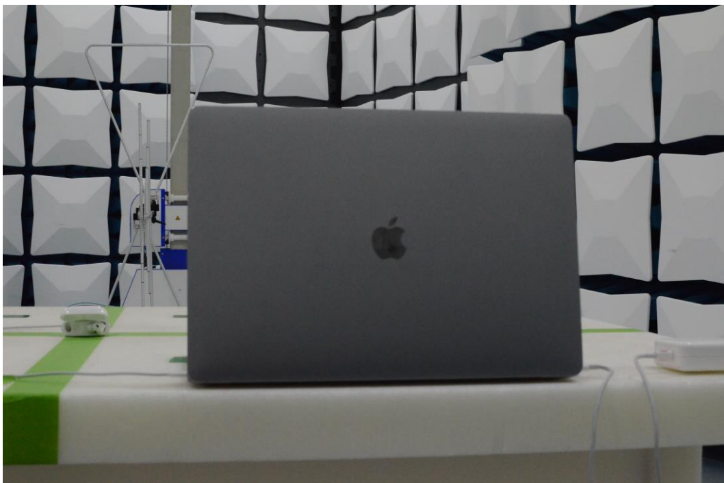
Figure 18: 30MHz-1GHz Test Setup (Rear View)
