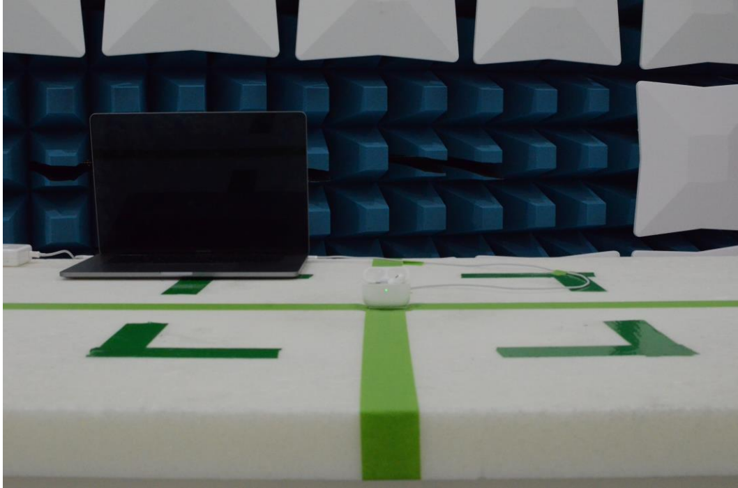
Figure 19: 30MHz-1GHz Test Setup (Front View)
