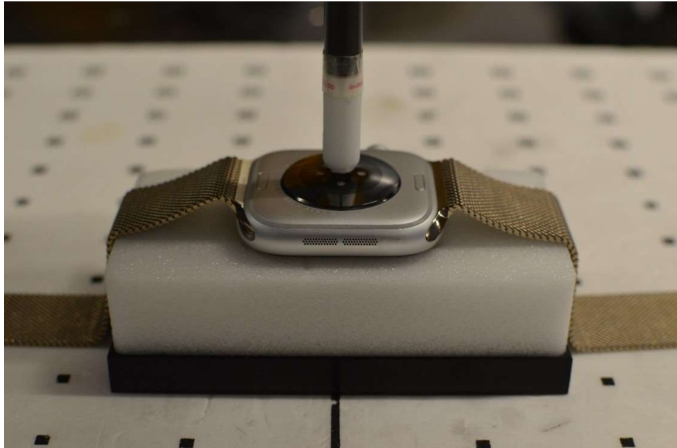
Near Field Power Density Test Setup Photo 21 – Aluminum with Metal Loop Wristband, Extremity, Back side at 2mm
