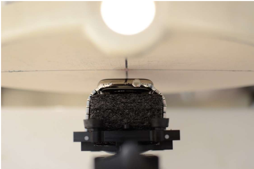
SAR Test Setup Photo 5 – Titanium with Metal Links Wristband, Head, Front side at 10 mm
