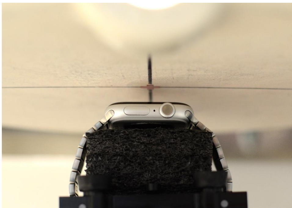
SAR Test Setup Photo 2 – Aluminum with Metal Links Wristband, Head, Front Side at 10mm
