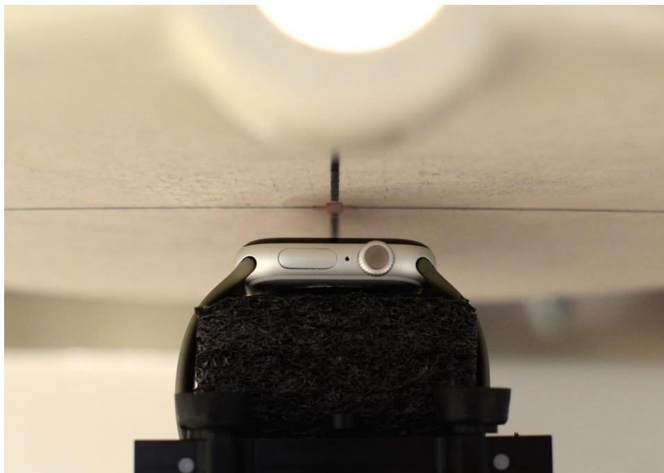
SAR Test Setup Photo 1 – Aluminum with Sport Wristband, Head, Front Side at 10mm
