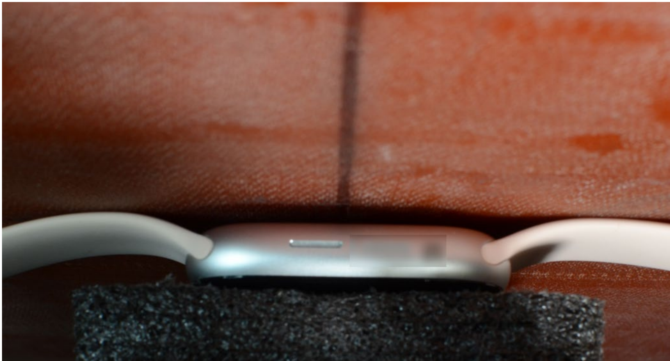
NFC Test Setup Photo 7: Aluminum with Sport Wristband, Extremity, Back Side at 0.0 cm
