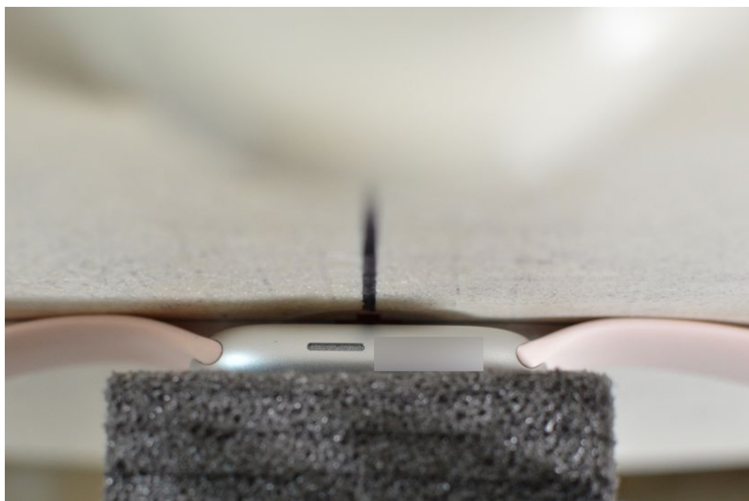
SAR Test Setup Photo 4: Aluminum with Sport Wristband, Extremity, Back Side at 0.0 cm
