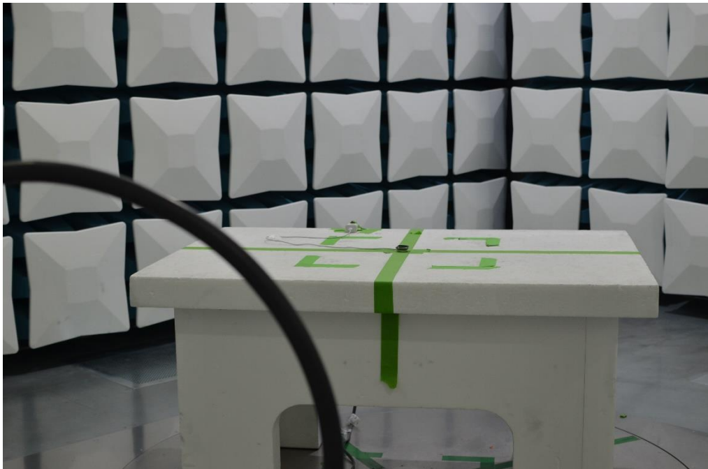
Figure 23: 9kHz-30MHz Test Setup (Front View)
