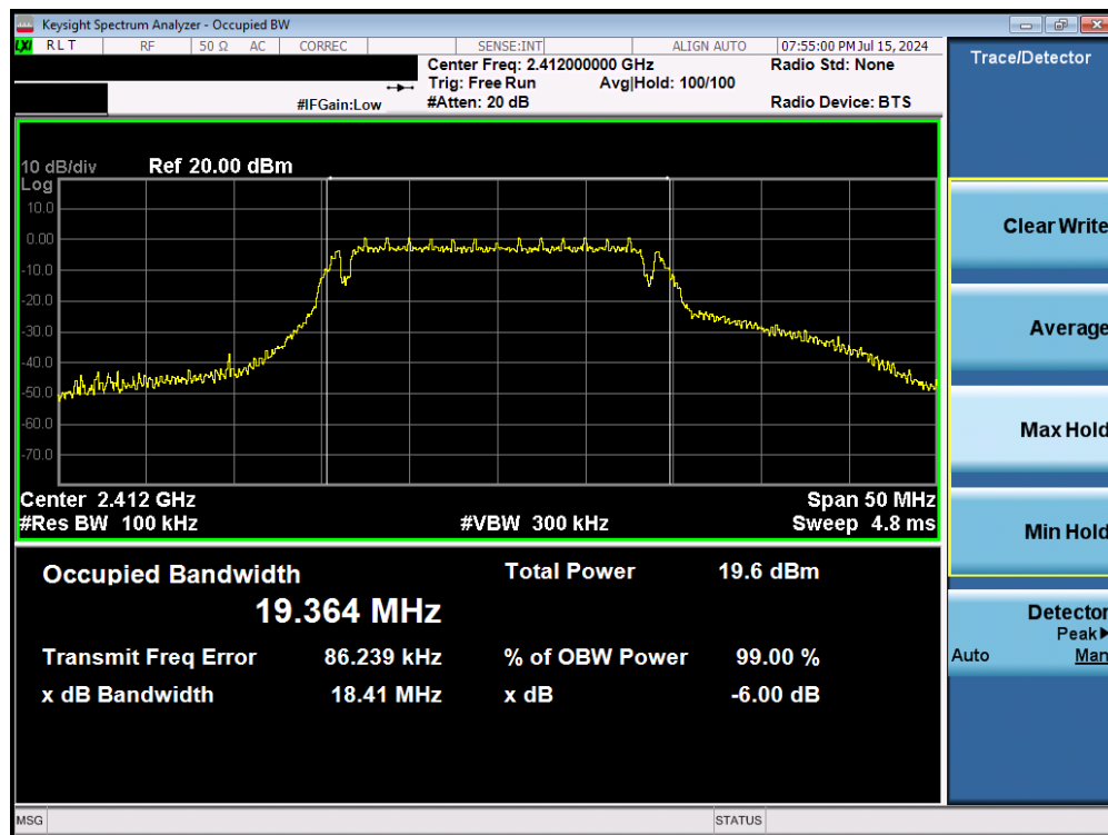
Plot 7-4. 6 dB BW and 99% OBW Plot (802.11g – Ch. 1) – 6Mbps
