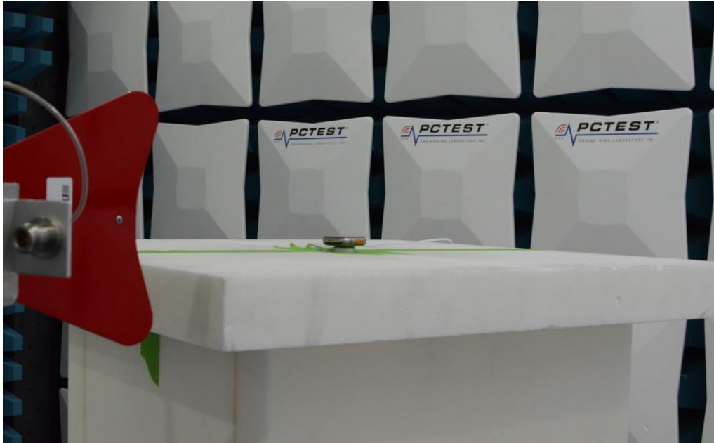
Figure 5: Above 960MHz Test Setup
