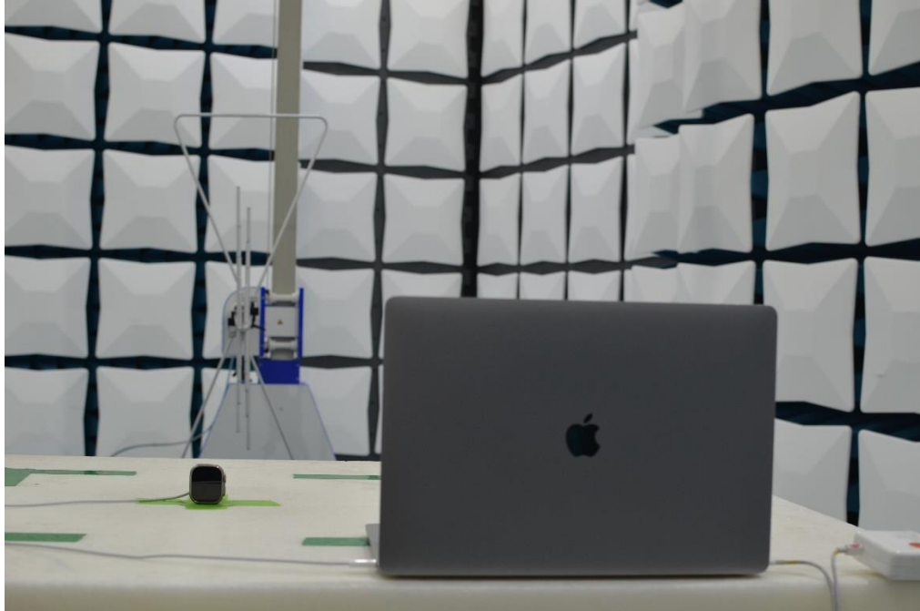
Figure 19: 30MHz-1GHz Test Setup (Rear View)
