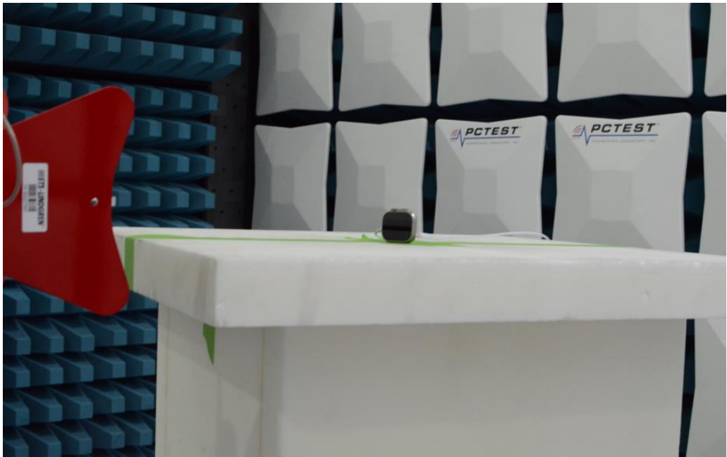
Figure 6: Above 960MHz Test Setup
