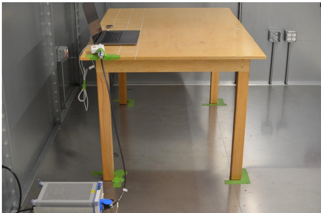
Figure 4: AC Line Conducted Emissions (Side View)
