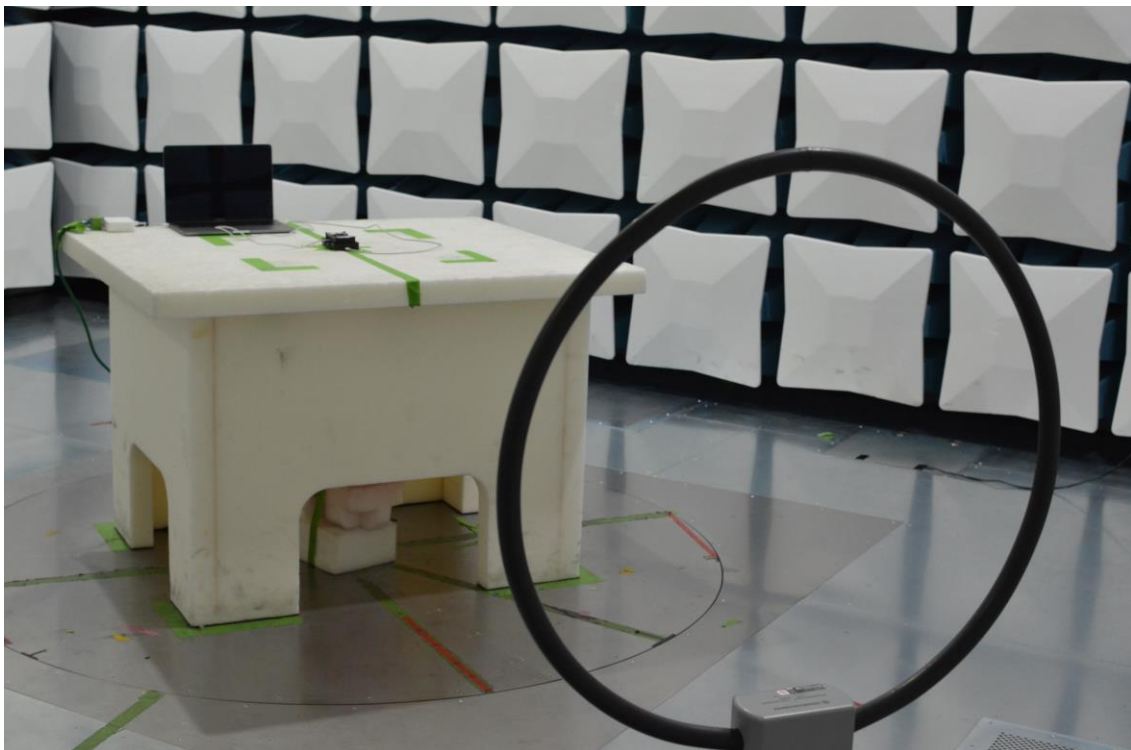
Figure 18: 9kHz-30MHz Test Setup (Front View)
