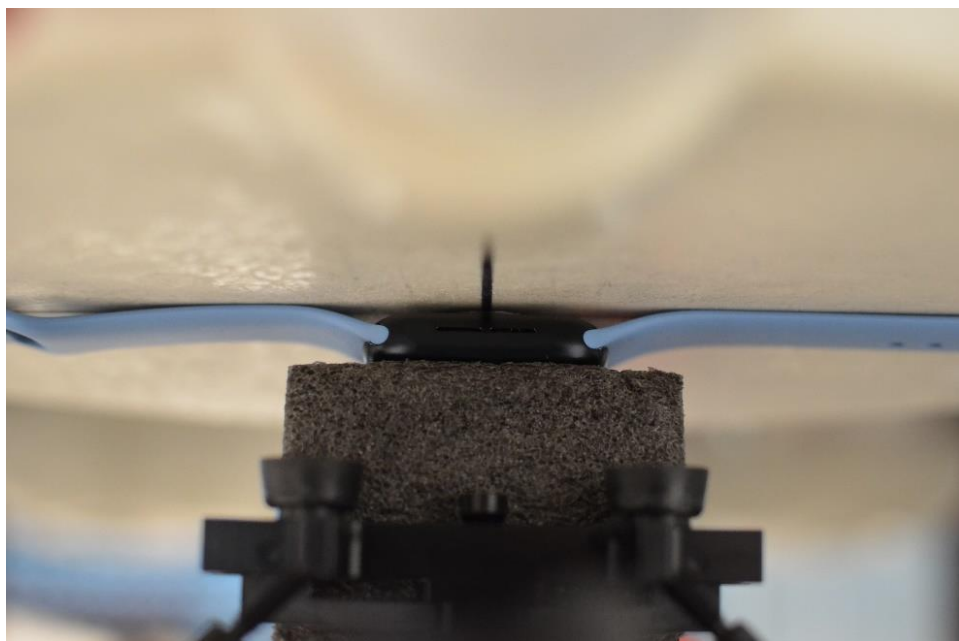
SAR Test Setup Photo 4: Aluminum with Sport Wristband, Extremity, Back Side at 0 mm
