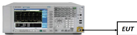
Figure 7-5. Test Instrument & Measurement Setup
