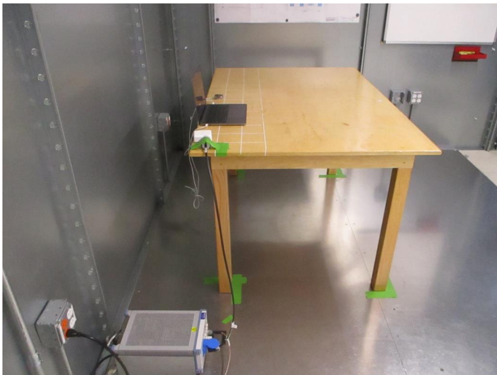
Figure 4: AC Line Conducted Emissions (Side View)
