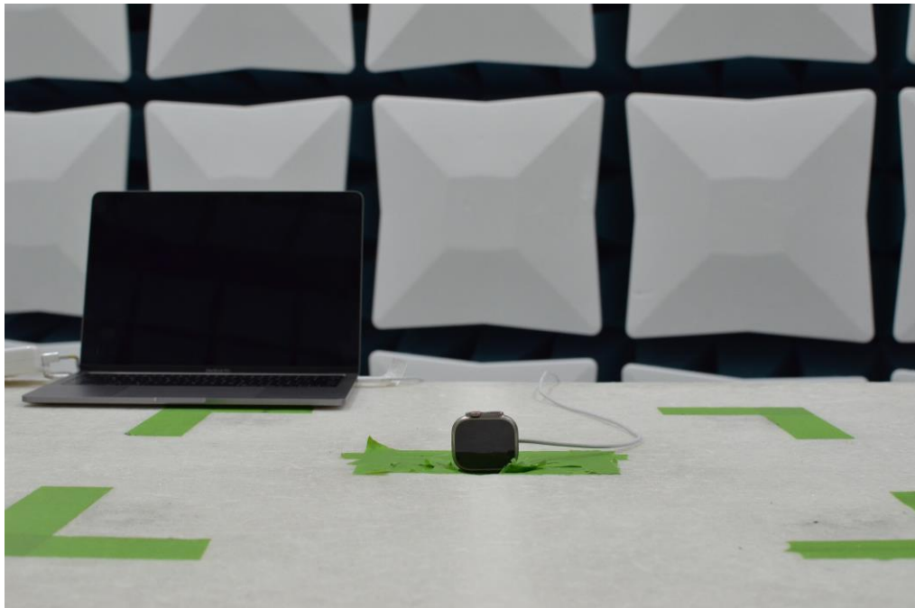
Figure 19: 30MHz-1GHz Test Setup (Front View)
