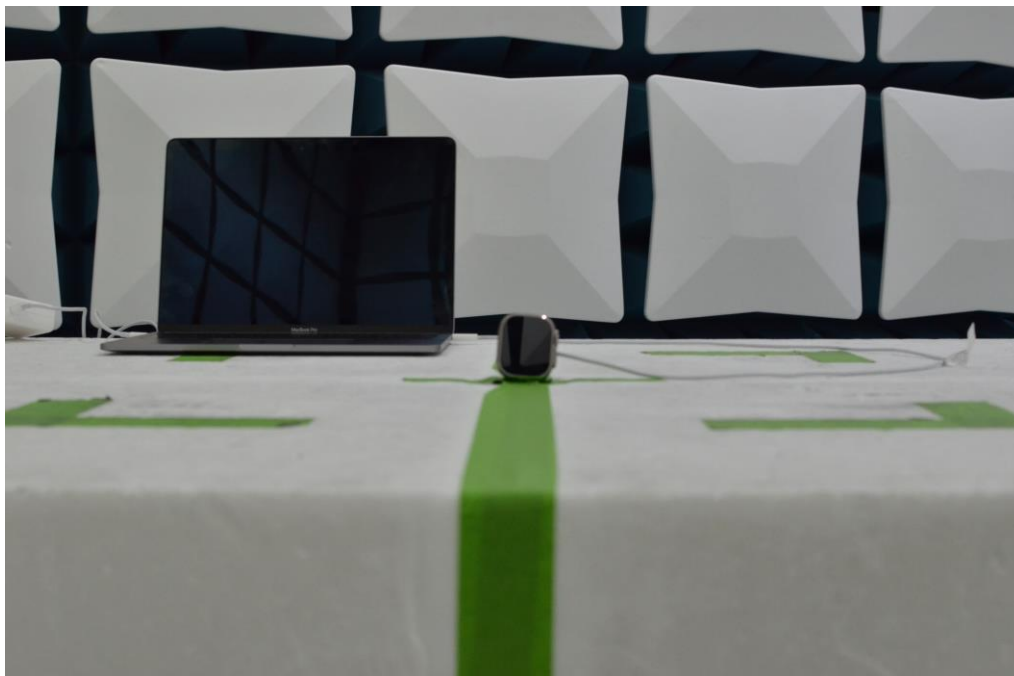
Figure 21: 30MHz-1GHz Test Setup (Front View)
