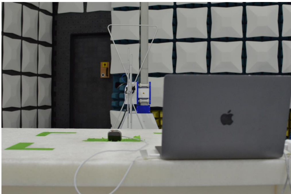
Figure 20: 30MHz-1GHz Test Setup (Rear View)
