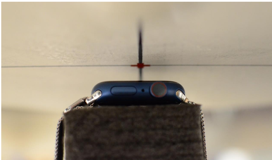
SAR Test Setup Photo 3: Head, Aluminum with Metal Loop Wristband, Front side at 1.0 cm
