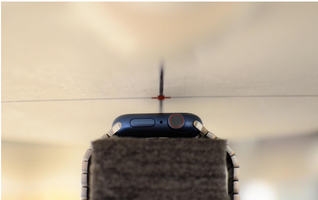
SAR Test Setup Photo 2: Head, Aluminum with Metal Links Wristband, Front side at 1.0 cm
