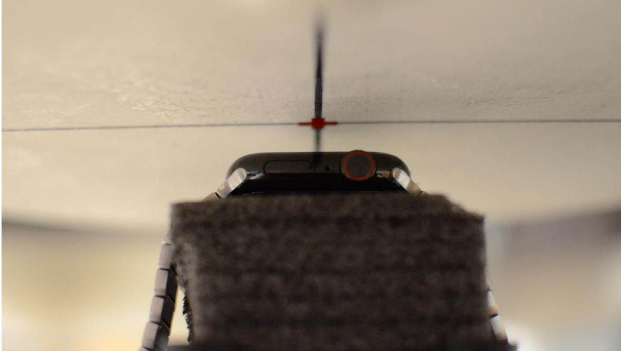
SAR Test Setup Photo 5: Head, Stainless Steel with Metal Links Wristband, Front side at 1.0 cm
