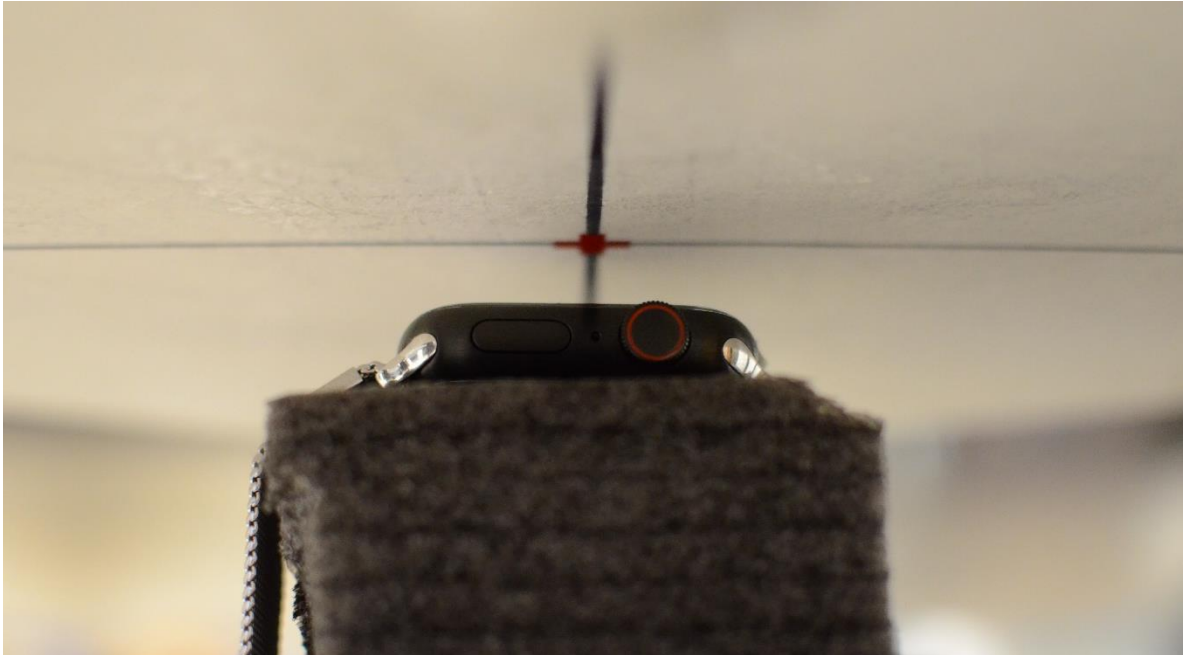
SAR Test Setup Photo 9: Head, Titanium with Metal Loop Wristband, Front side at 1.0 cm
