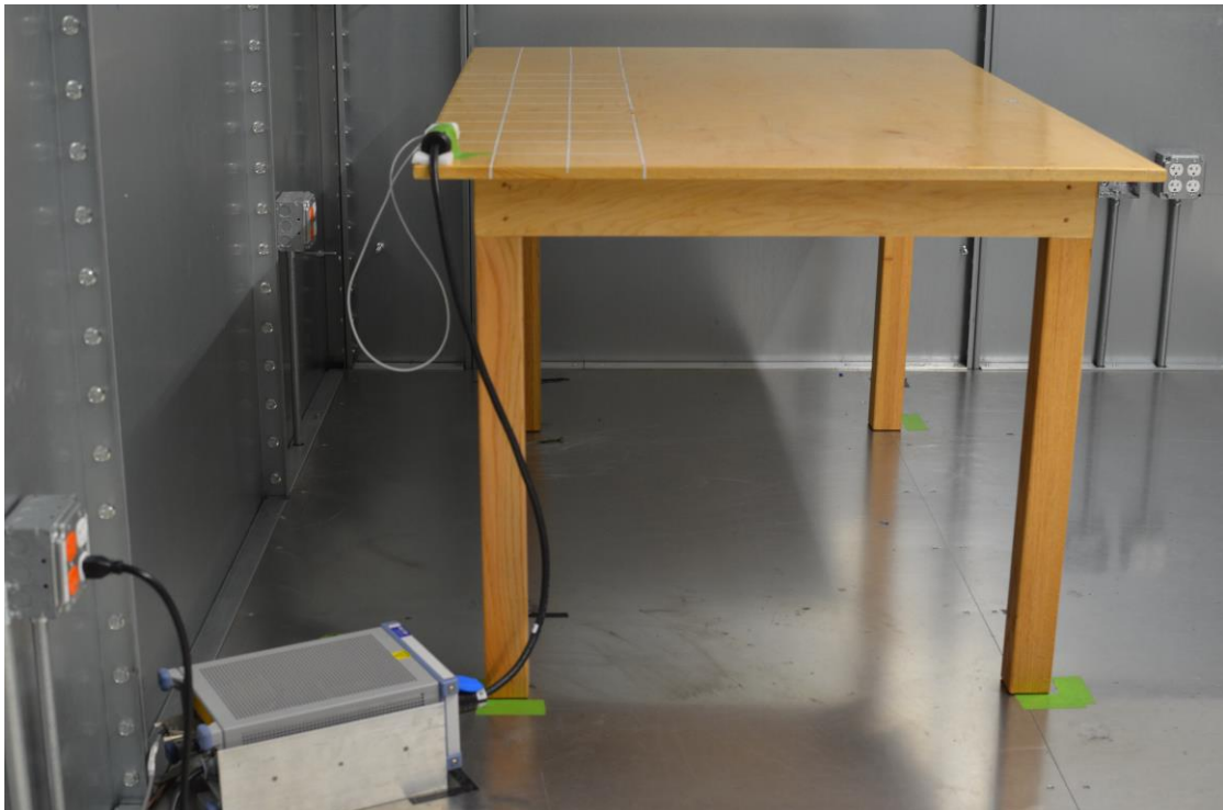
Figure 2: AC Line Conducted Emissions (Side View)
