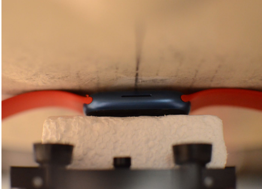
SAR Test Setup Photo 4: Aluminum with Sport Wrist Band, Extremity, Back Side at 0.0 cm
