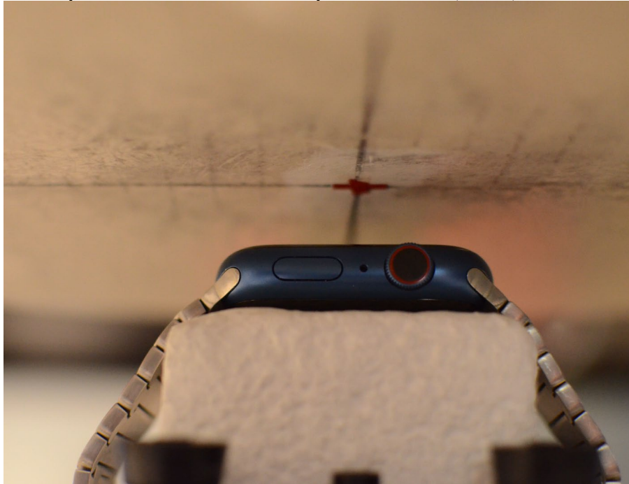
SAR Test Setup Photo 2: Aluminum with Metal Links Wrist Band, Head, Front Side at 1.0 cm
