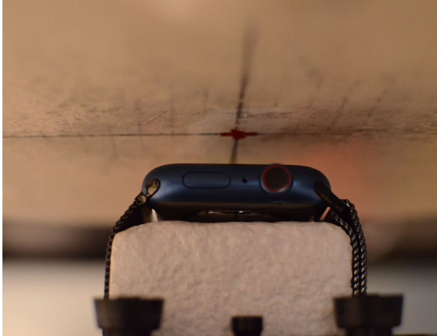
SAR Test Setup Photo 3: Aluminum with Metal Loop Wrist Band, Head, Front Side at 1.0 cm
