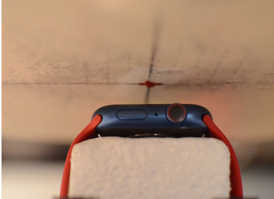
SAR Test Setup Photo 1: Aluminum with Sport Wrist Band, Head, Front Side at 1.0 cm
