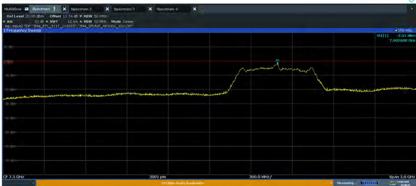
Plot 7-56. Peak Radiated Power (Ch. 9, Config 1/Payload 125)
