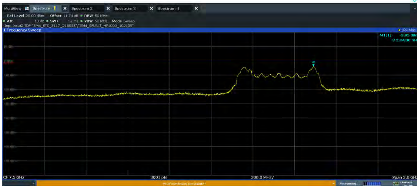
Plot 7-59. Peak Radiated Power (Ch. 9, Config 4/Payload 0)
