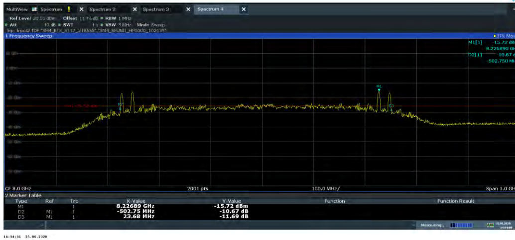
Plot 7-15. 10dBc Bandwidth (Ch. 9, Config 1/Payload 85)
