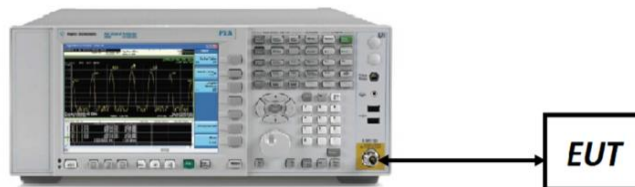
Figure 7-1. Test Instrument & Measurement Setup
