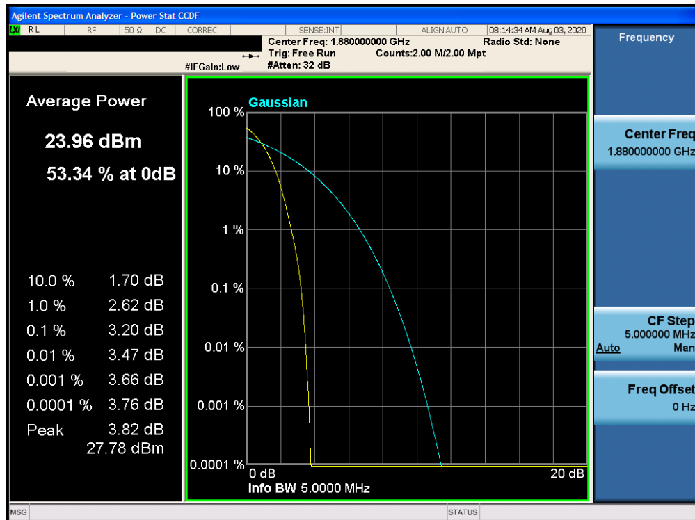
Plot 7-43. Peak-Average Ratio Plot (PCS WCDMA Mode)
