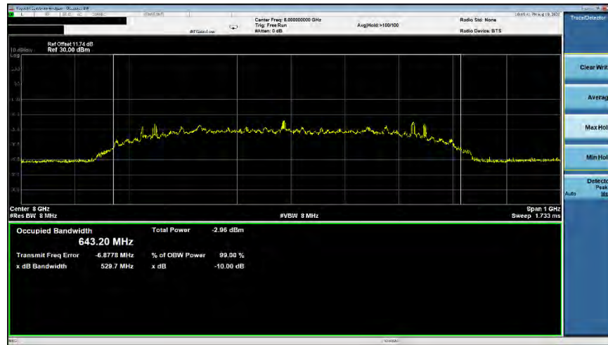
Plot 7-37. ISED Occupied Bandwidth (Ch. 9, Config 2/Payload 125)
