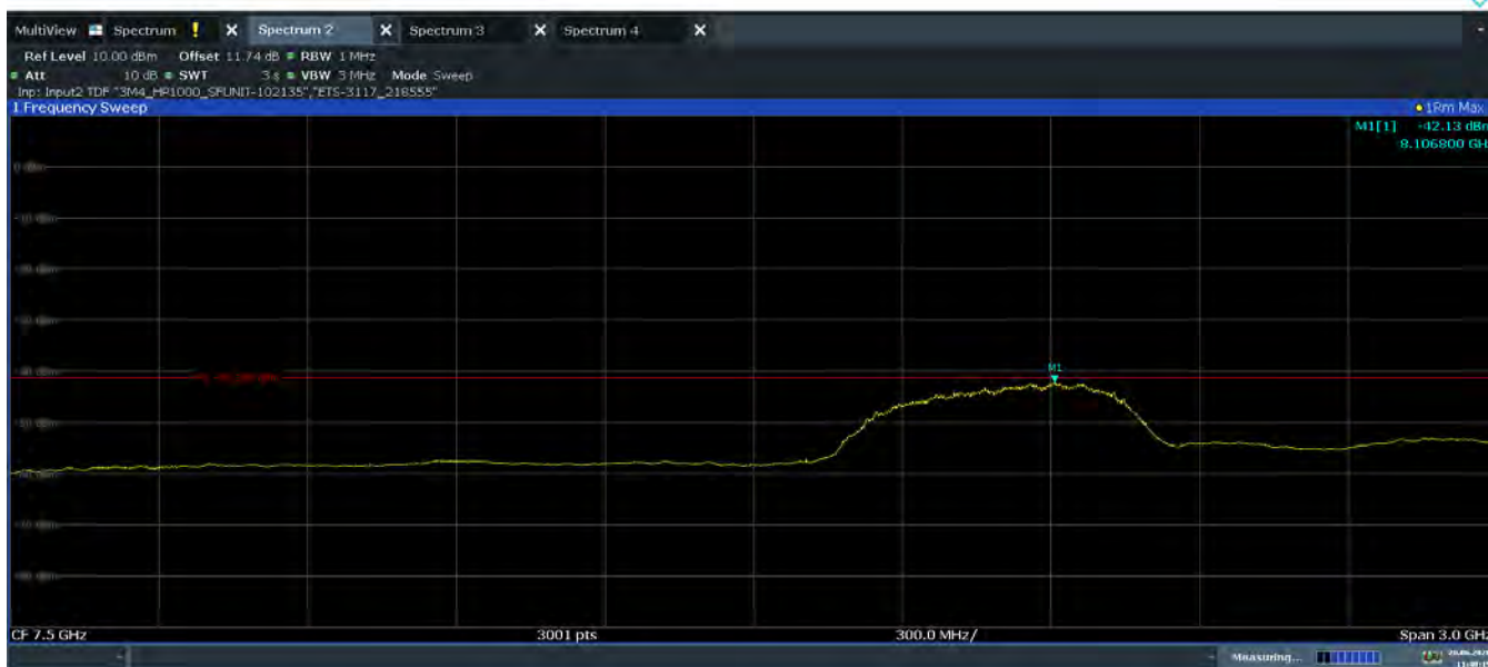
Plot 7-79. Average Radiated Power (Ch. 9, Config 4/Payload 0)
