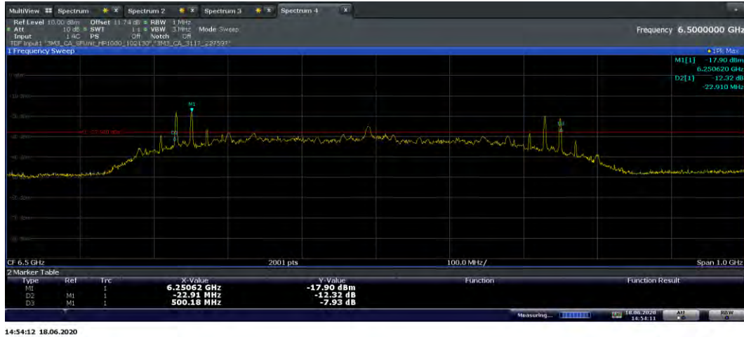
Plot 7-7. 10dBc Bandwidth (Ch. 5, Config 2/Payload 125)
