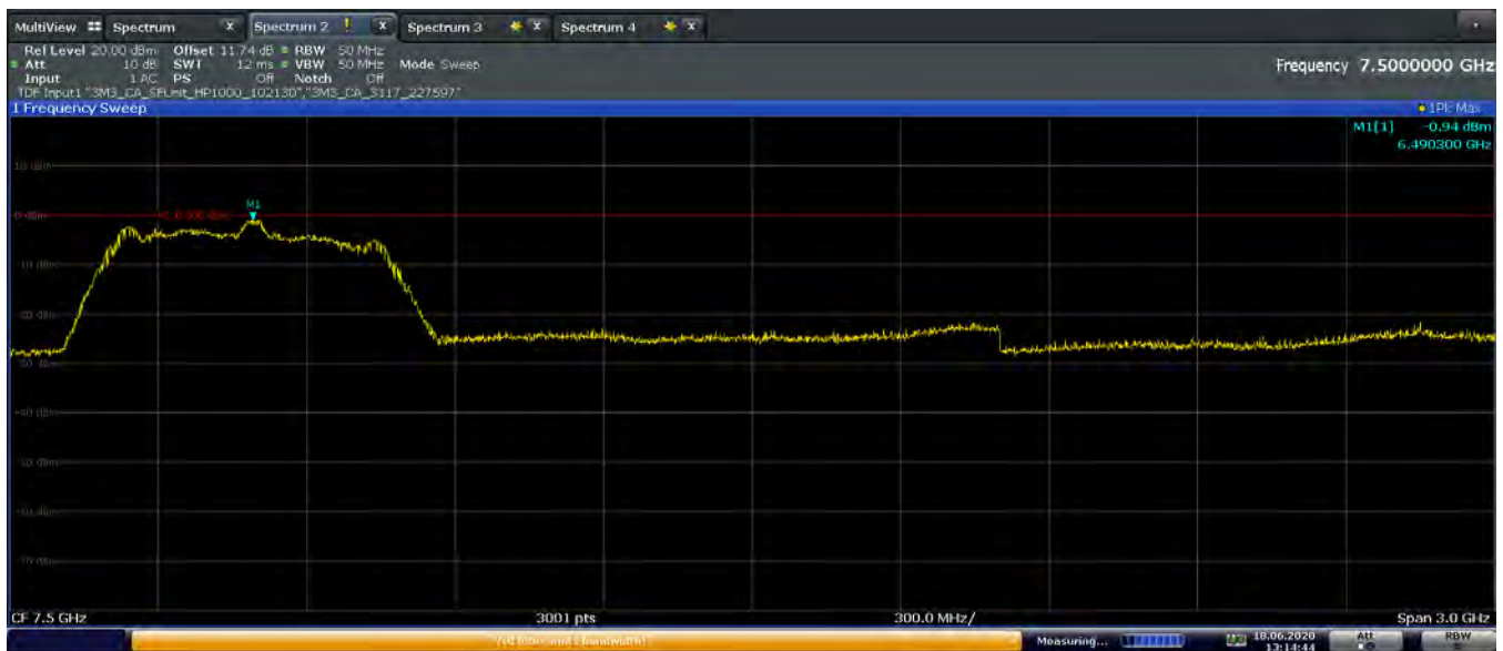
Plot 7-44. Peak Radiated Power (Ch. 5, Config 1/Payload 45)
