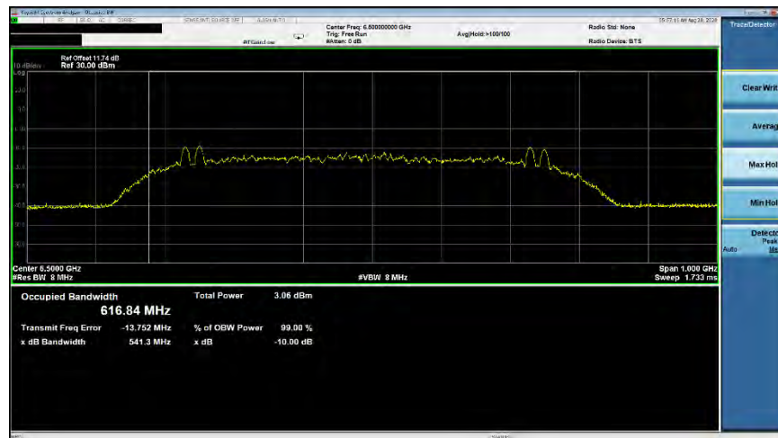
Plot 7-23. ISSED Occupied Bandwidth (Ch. 5, Config 0/Payload 125)
