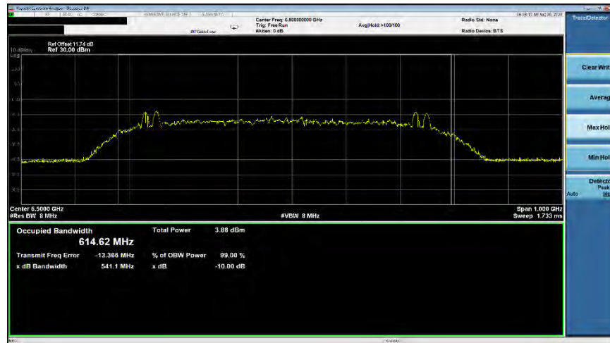
Plot 7-22. ISSED Occupied Bandwidth (Ch. 5, Config 0/Payload 65)
