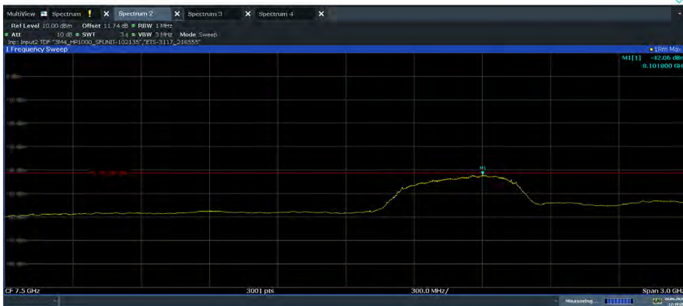
Plot 7-80. Average Radiated Power (Ch. 9, Config 5/Payload 0)
