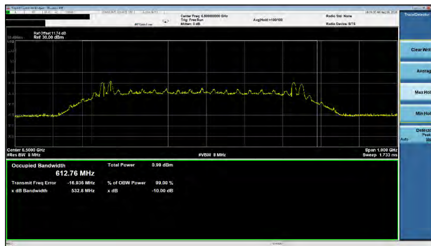
Plot 7-29. ISSED Occupied Bandwidth (Ch. 5, Config 4/Payload 0)
