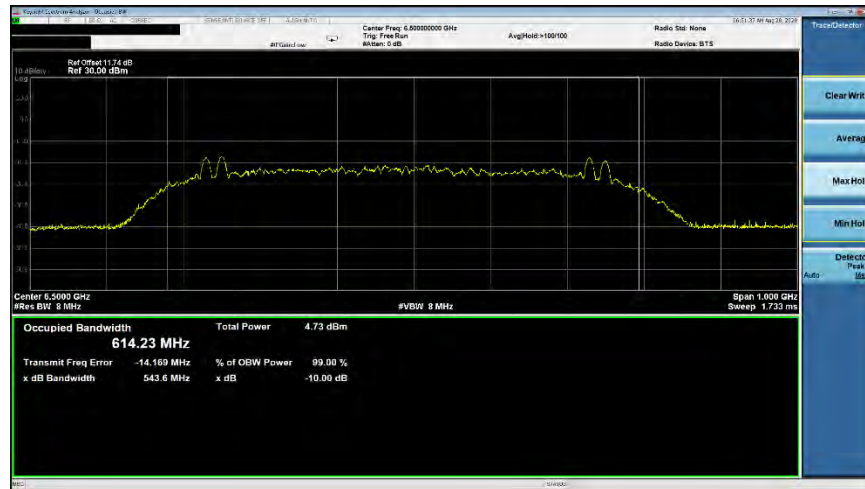
Plot 7-21. ISSED Occupied Bandwidth (Ch. 5, Config 0/Payload 25)
