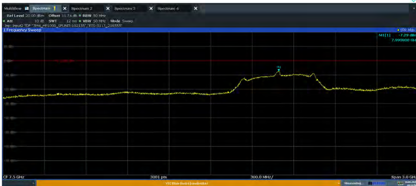
Plot 7-57. Peak Radiated Power (Ch. 9, Config 2/Payload 125)
