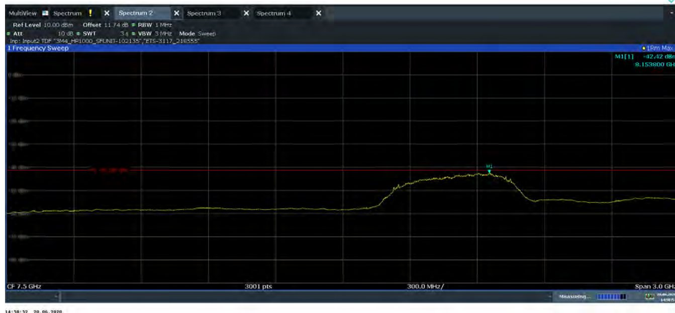
Plot 7-71. Average Radiated Power (Ch. 9, Config 0/Payload 25)
