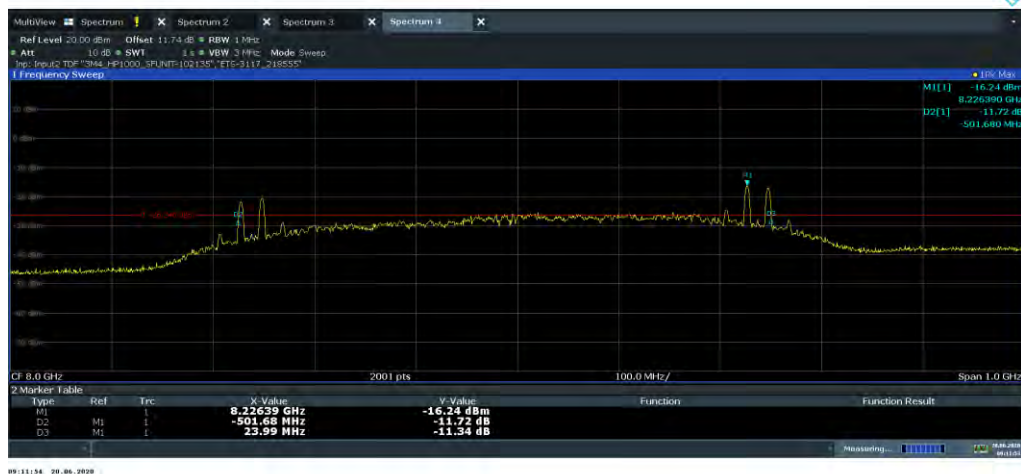
Plot 7-16. 10dBc Bandwidth (Ch. 9, Config 1/Payload 125)
