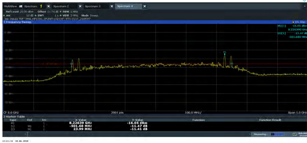
Plot 7-15. 10dBc Bandwidth (Ch. 9, Config 1/Payload 85)
