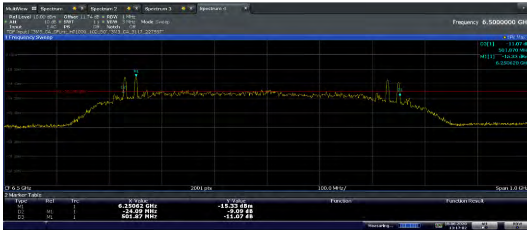
Plot 7-4. 10dBc Bandwidth (Ch. 5, Config 1/Payload 45)
