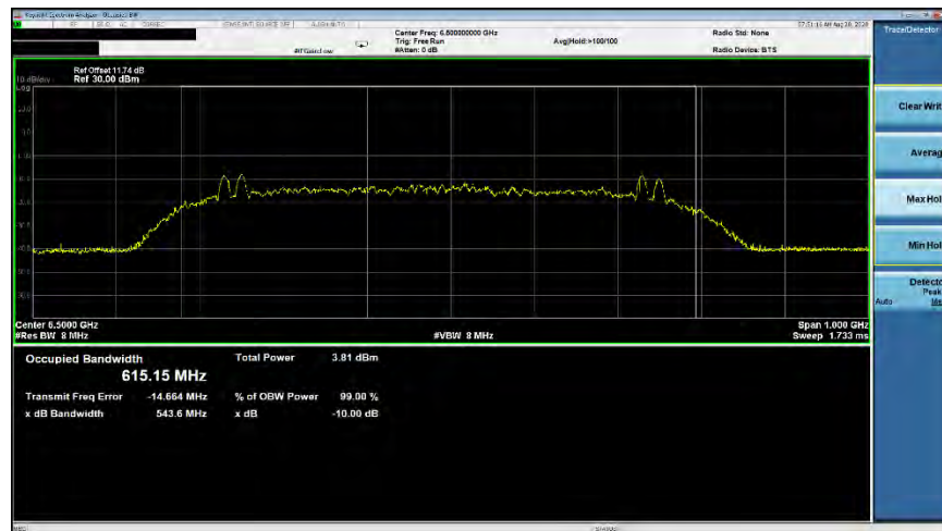
Plot 7-25. ISED Occupied Bandwidth (Ch. 5, Config 1/Payload 85)
