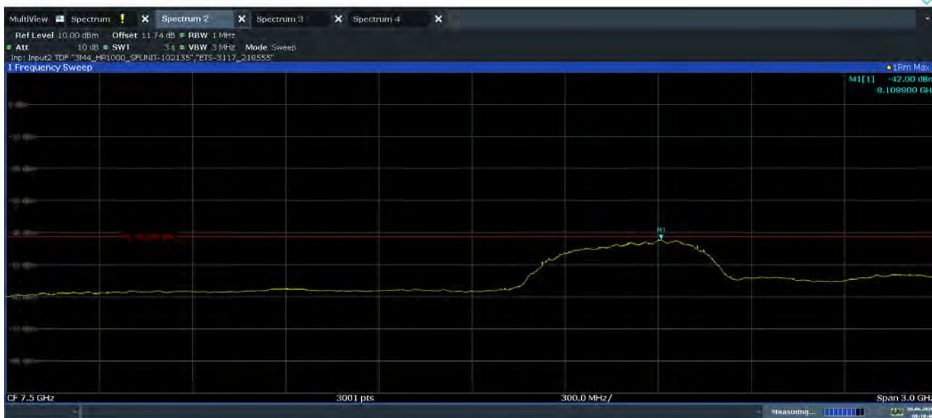
Plot 7-77. Average Radiated Power (Ch. 9, Config 2/Payload 125)
