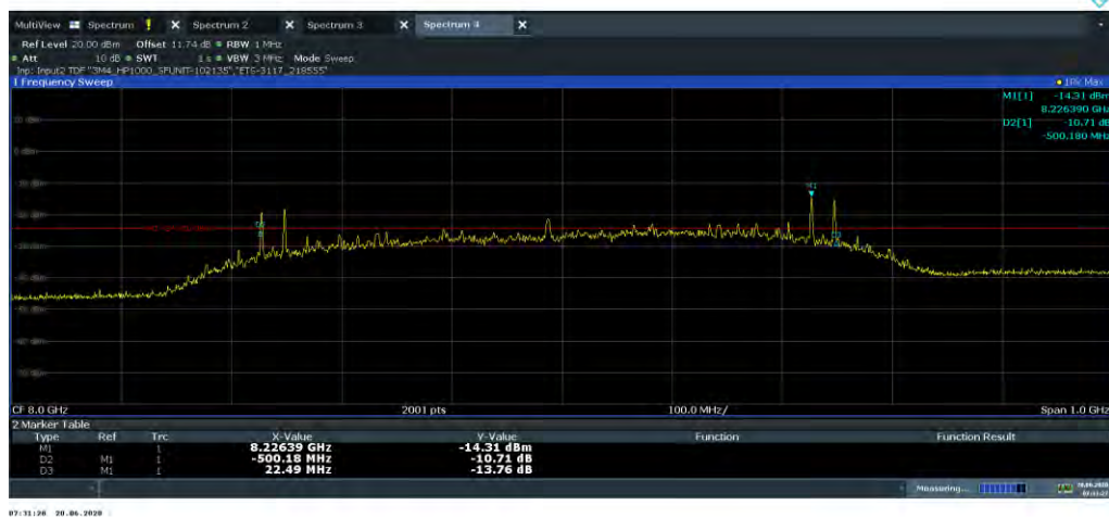
Plot 7-18. 10dBc Bandwidth (Ch. 9, Config 3/Payload 125)
