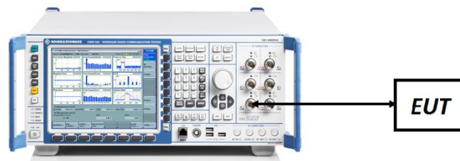
Figure 7-4. Conducted Power Measurement Setup
