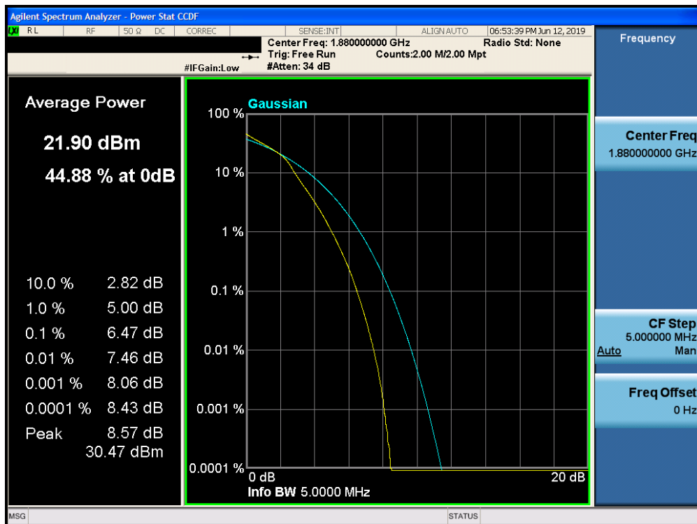
Plot 7-297. PAR Plot (Band 2 - 5.0MHz 16-QAM - Full RB Configuration)
