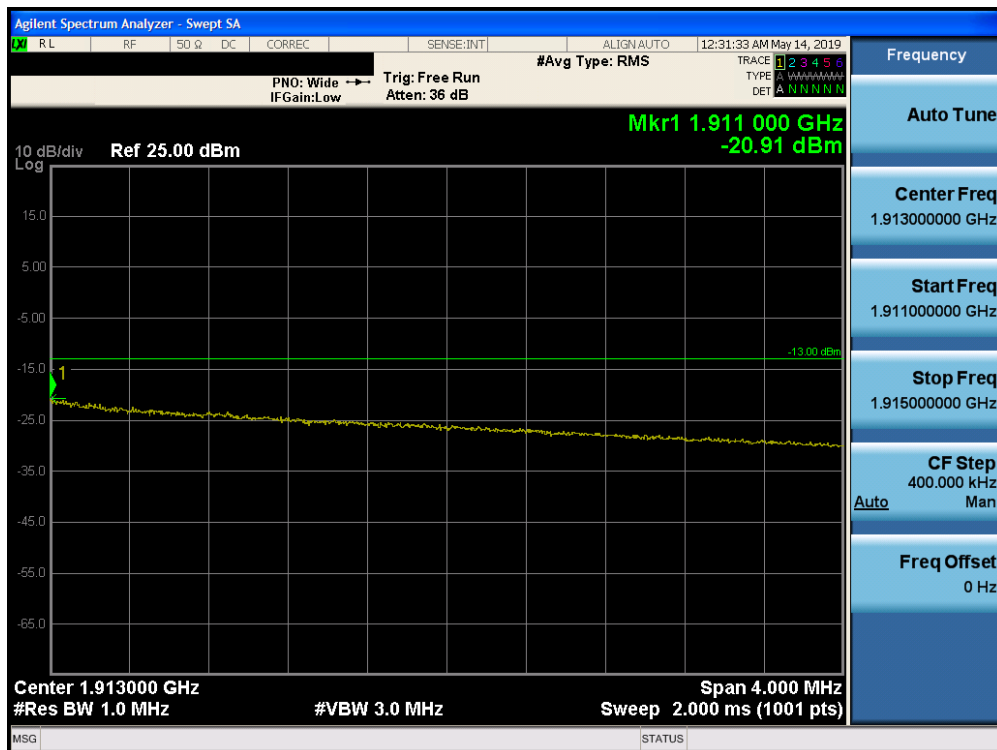
Plot 7-243. Upper Extended Band Edge Plot (Band 2 - 10.0MHz QPSK - Full RB Configuration)
