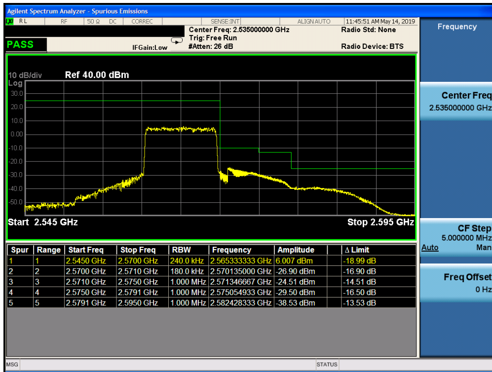
Plot 7-255. Upper ACP Plot (Band 7 - 10.0MHz QPSK - Full RB Configuration)
