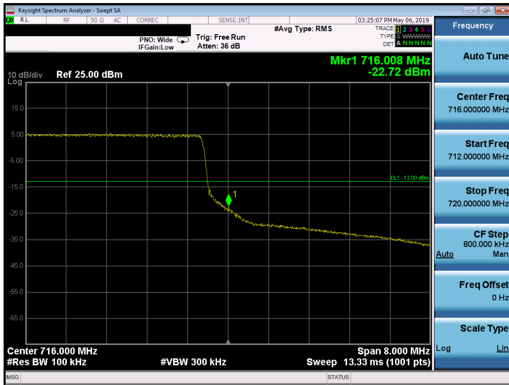
Plot 7-135. Upper Band Edge Plot (Band 17 - 10.0MHz QPSK - Full RB Configuration)
