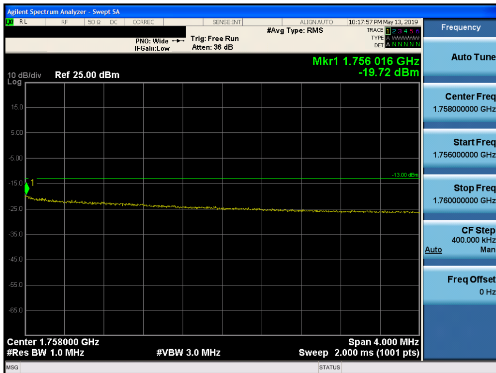
Plot 7-195. Upper Extended Band Edge Plot (Band 4 - 10.0MHz QPSK - Full RB Configuration)
