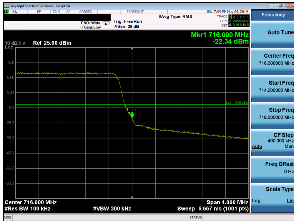
Plot 7-133. Upper Band Edge Plot (Band 17 - 5.0MHz QPSK - Full RB Configuration)
