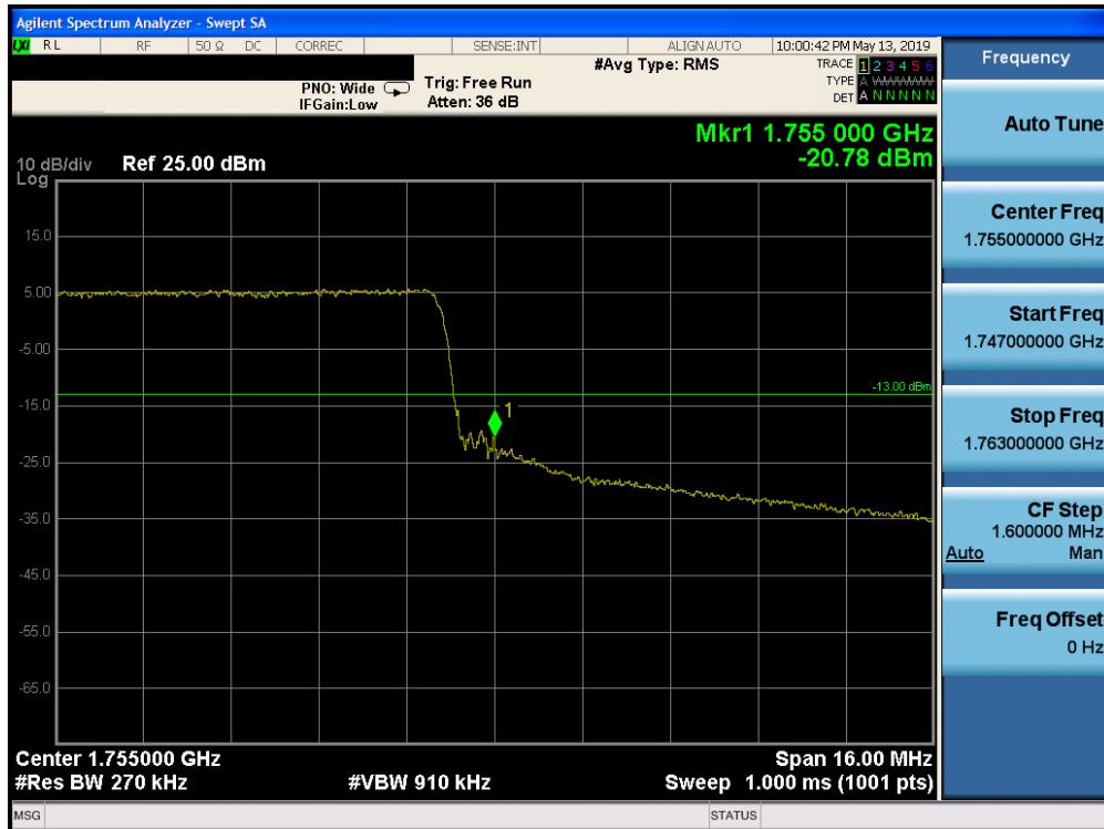
Plot 7-202. Upper Band Edge Plot (Band 4 - 20.0MHz QPSK - Full RB Configuration)
