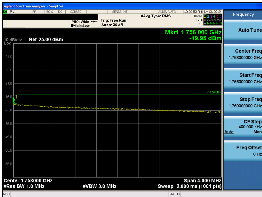
Plot 7-203. Upper Extended Band Edge Plot (Band 4 - 20.0MHz QPSK - Full RB Configuration)
