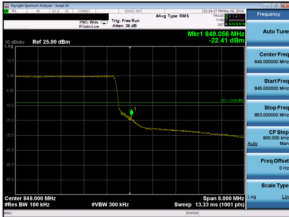
Plot 7-155. Upper Band Edge Plot (Band 5 - 10.0MHz QPSK - Full RB Configuration)
