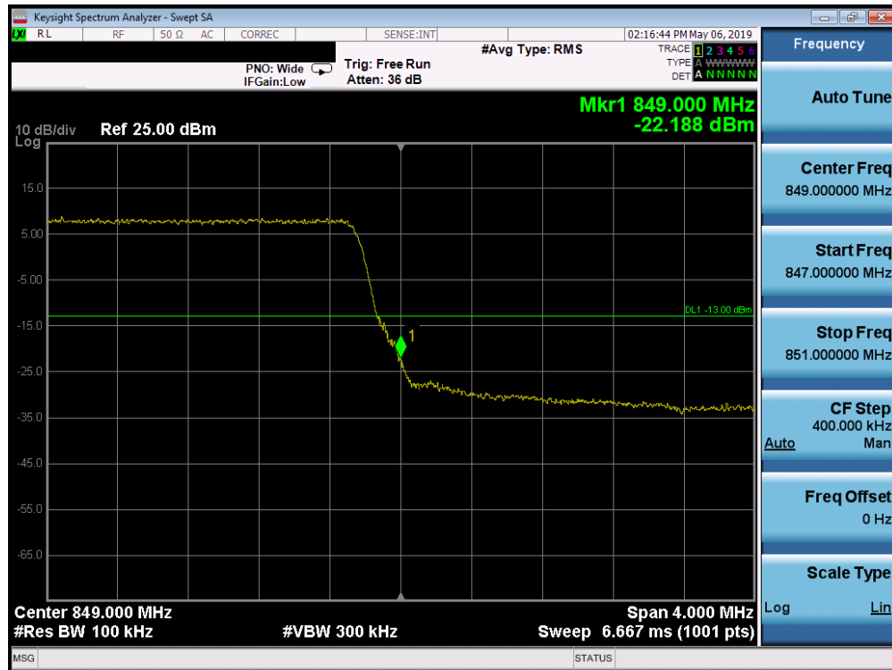
Plot 7-153. Upper Band Edge Plot (Band 5 - 5.0MHz QPSK - Full RB Configuration)
