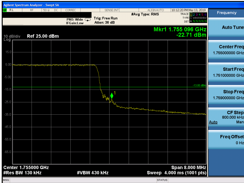
Plot 7-194. Upper Band Edge Plot (Band 4 - 10.0MHz QPSK - Full RB Configuration)
