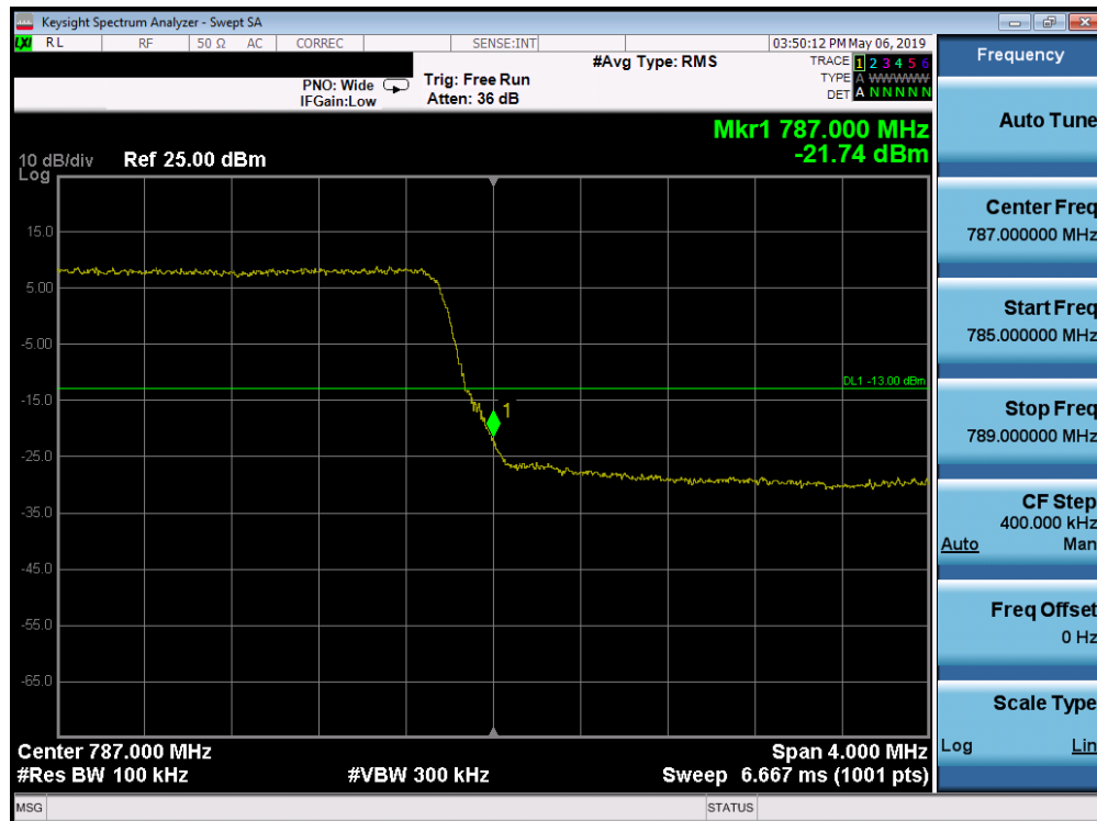
Plot 7-137. Upper Band Edge Plot (Band 13 - 5.0MHz QPSK - Full RB Configuration)
