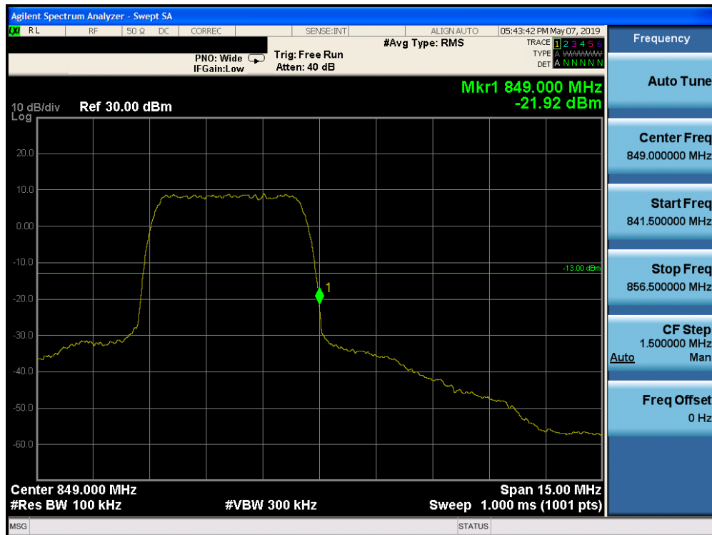
Plot 7-32. Band Edge Plot (Cellular WCDMA Mode - High Channel)
