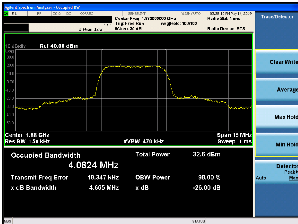
Plot 7-3. Occupied Bandwidth Plot (PCS WCDMA Mode)
