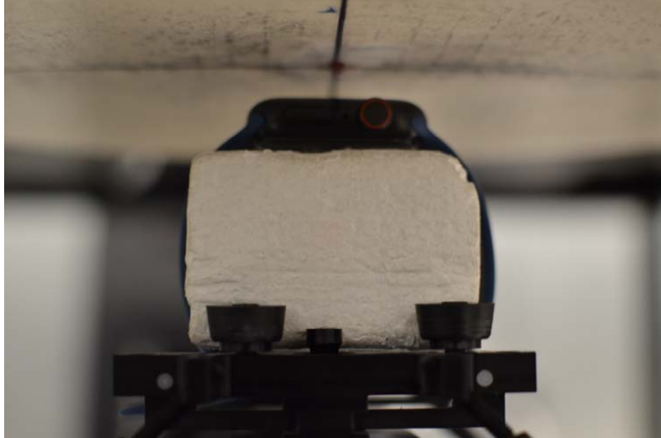
SAR Test Setup Photo 7: Titanium with Sport Wristband, Front side at 1.0 cm
