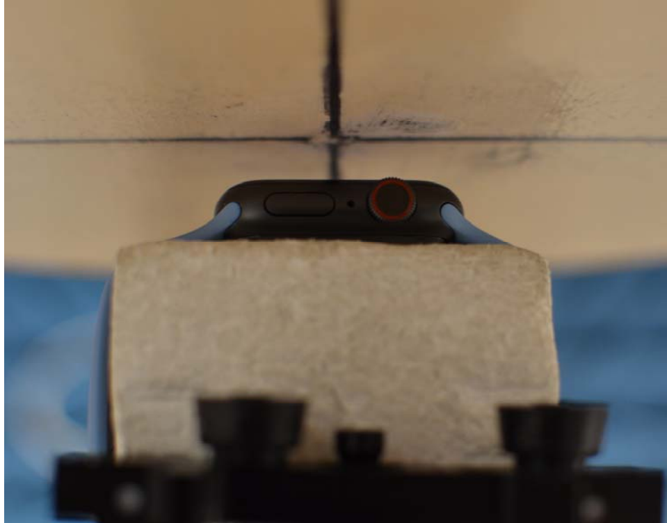
SAR Test Setup Photo 1: Aluminum with Sport Wristband, Front side at 1.0 cm
