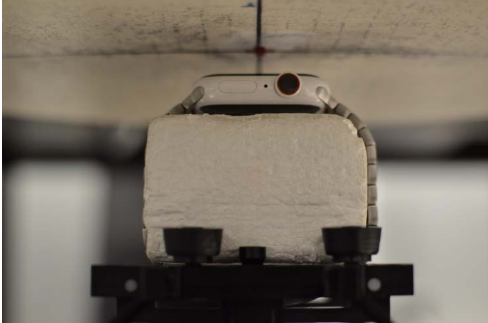
SAR Test Setup Photo 11: Ceramic with Metal Links Wristband, Front side at 1.0 cm
