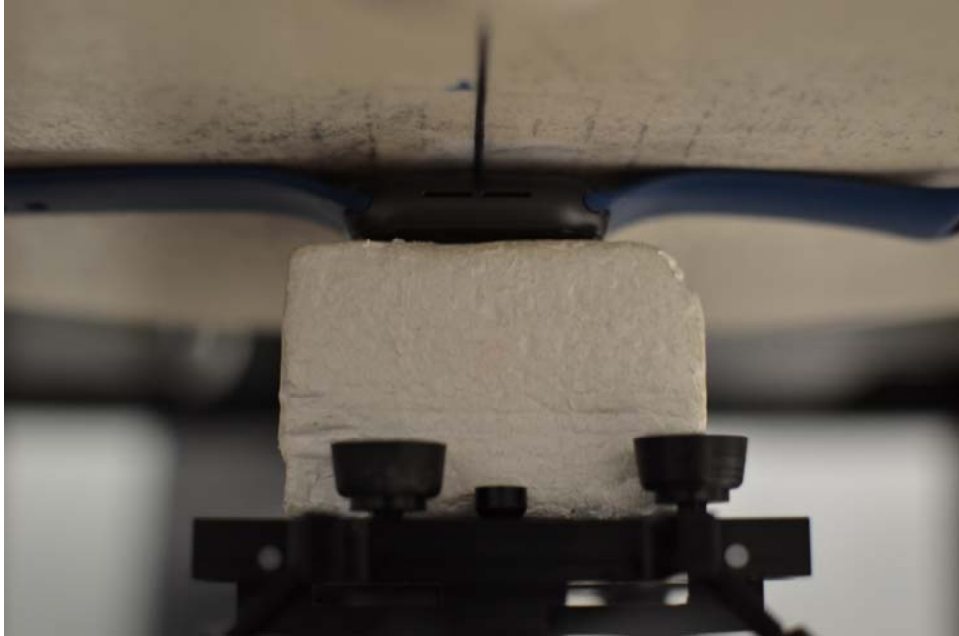
SAR Test Setup Photo 13: Aluminum with Sport Wristband, Back side at 0.0 cm
