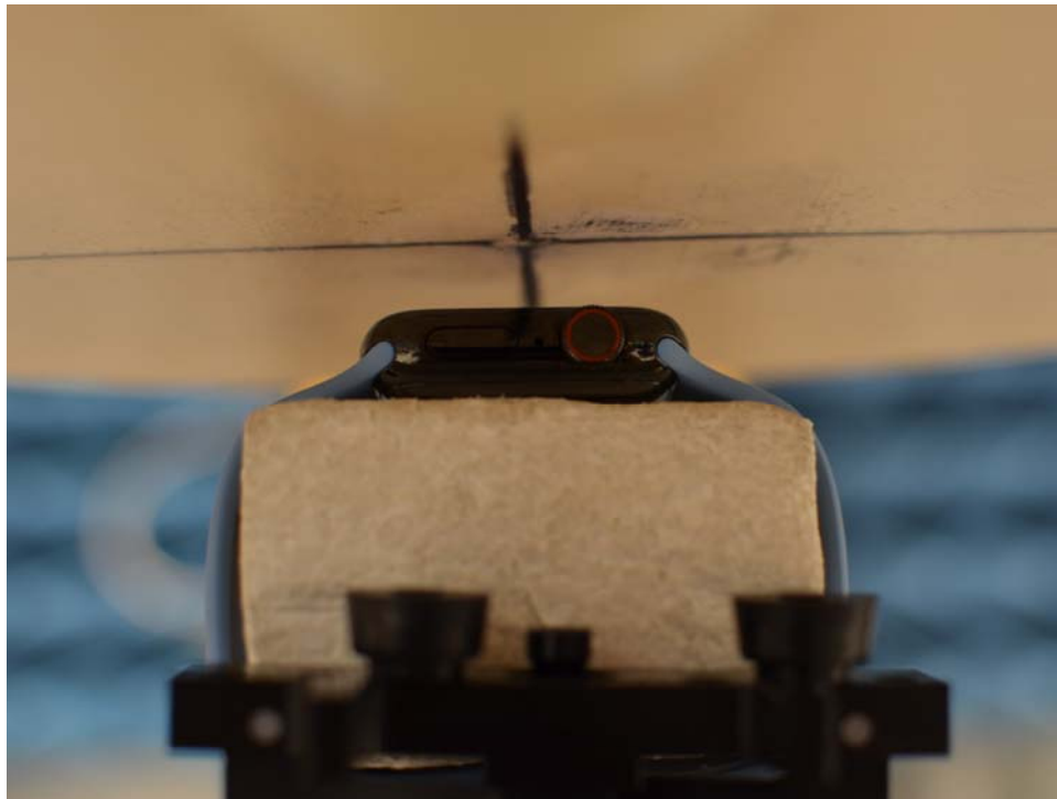
SAR Test Setup Photo 4: Stainless Steel with Sport Wristband, Front side at 1.0 cm
