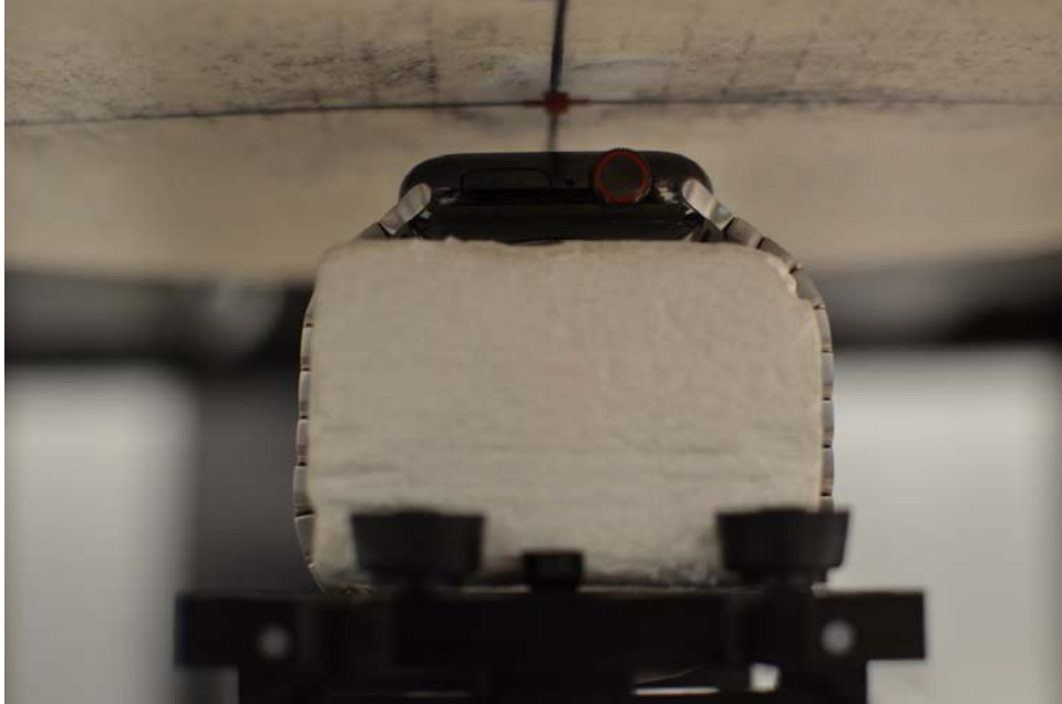
SAR Test Setup Photo 5: Stainless Steel with Metal Links Wristband, Front side at 1.0 cm
