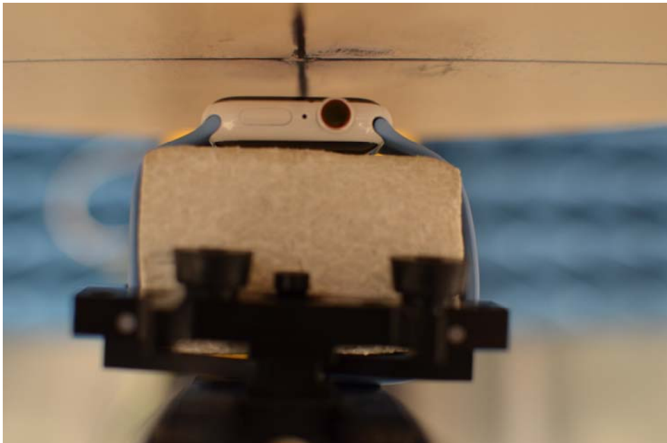
SAR Test Setup Photo 10: Ceramic with Sport Wristband, Front side at 1.0 cm
