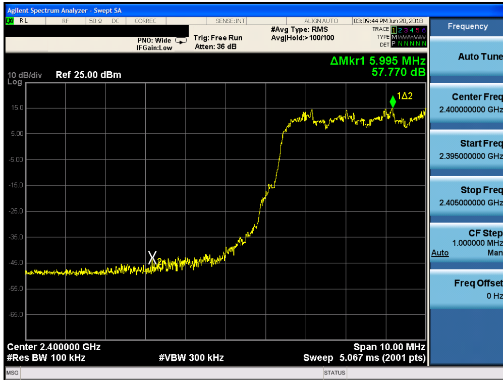
Plot 7-35. Band Edge Plot (Bluetooth with Hopping Enabled, 8DPSK, ePA)
