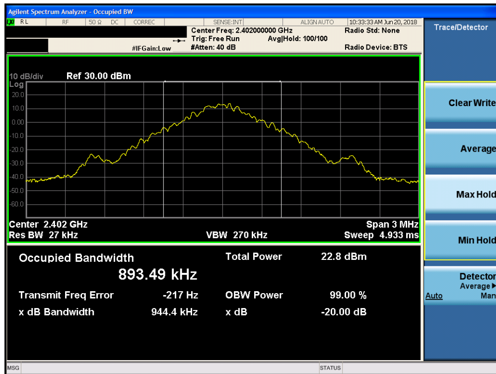
Plot 7-1. 20dB Bandwidth Plot (Bluetooth, GFSK, ePA – Ch. 0)
