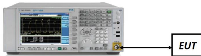
Figure 7-1. Test Instrument & Measurement Setup
