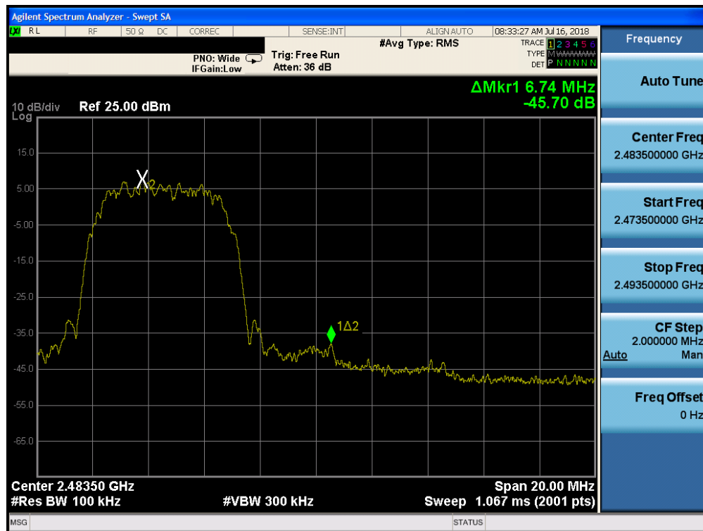
Plot 7-32. Band Edge Plot (Bluetooth (HDR, iPA), 8Mbps - Ch. 75)
