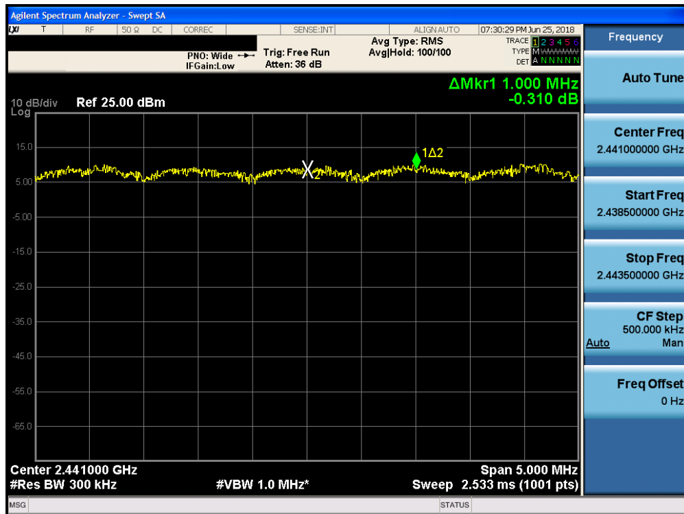
Plot 7-30. Channel Spacing Plot (Bluetooth, 8DPSK, ePA)
