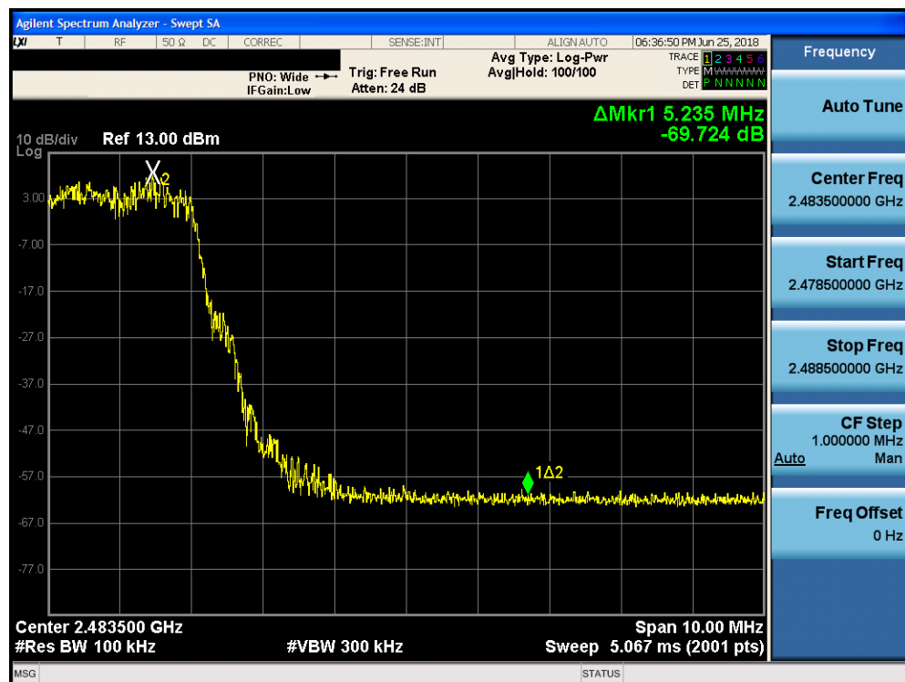
Plot 7-24. Band Edge Plot (Bluetooth with Hopping Enabled, 8DPSK, ePA – Ch. 78)
