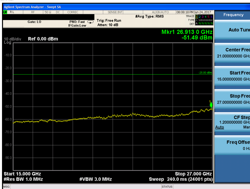
Plot 7-11. Conducted Spurious Plot (Band 41 – 10.0MHz QPSK – RB Size 1, RB Offset 0 – Low Channel)
