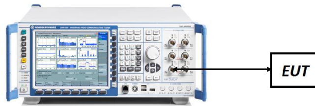
Figure 7-4. EIRP Measurement Setup
