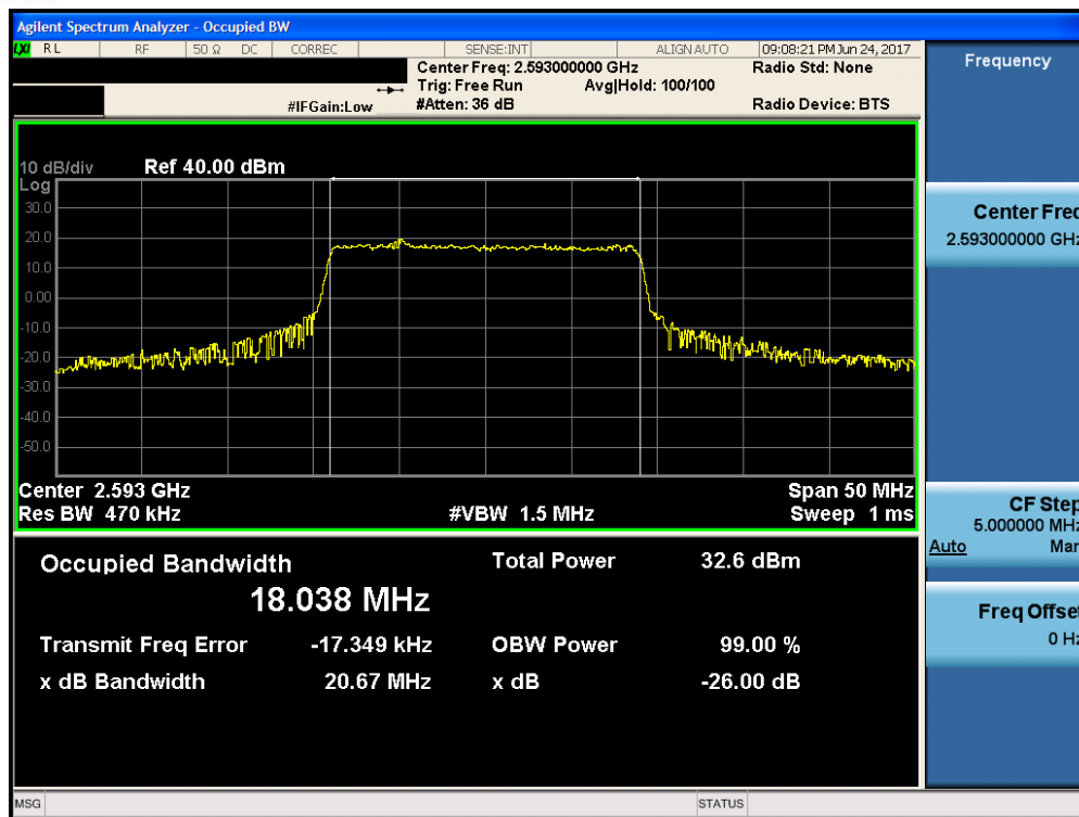
Plot 7-7. Occupied Bandwidth Plot (Band 41 – 20.0MHz QPSK – RB Size 100)
