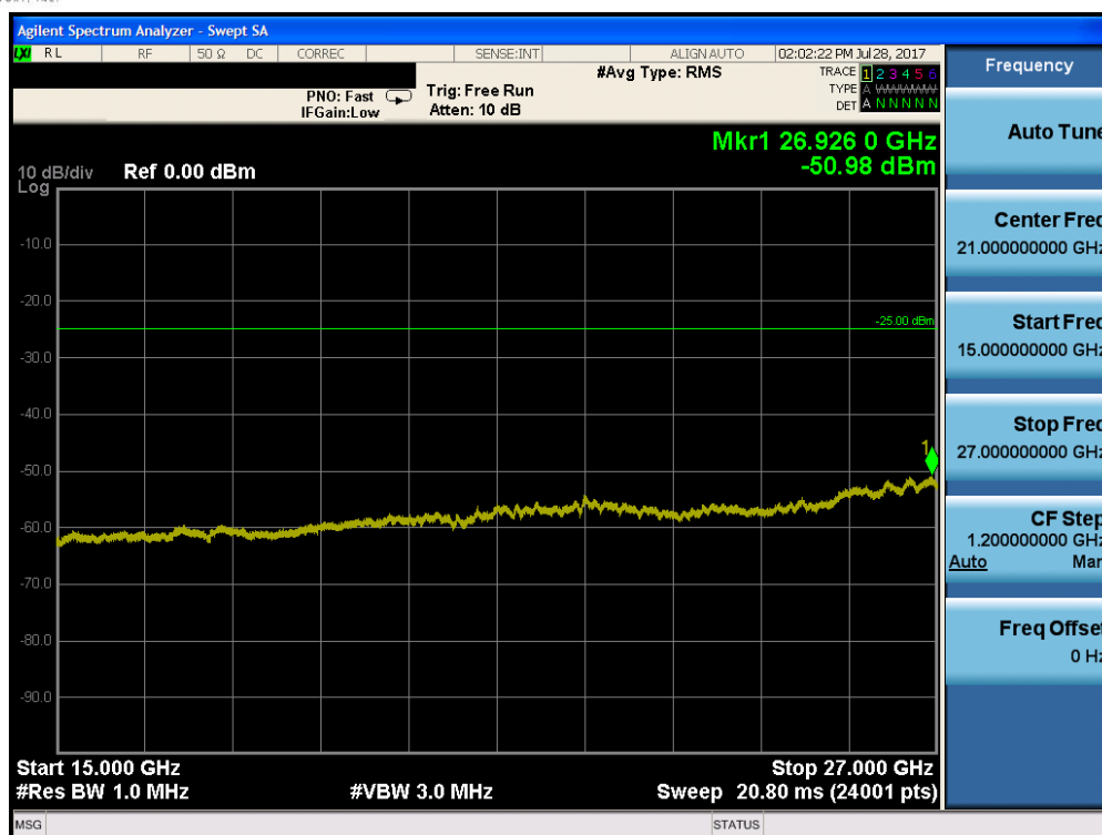
Plot 7-31. Conducted Spurious Plot (Band 7 – 5.0MHz QPSK – RB Size 1, RB Offset 0 – Mid Channel)
