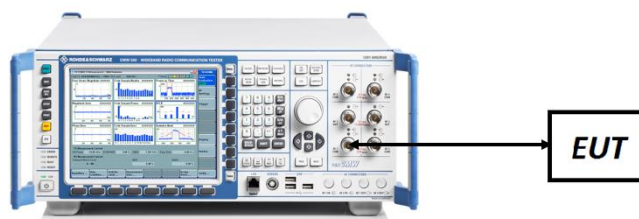
Figure 7-4. ERP/EIRP Measurement Setup
