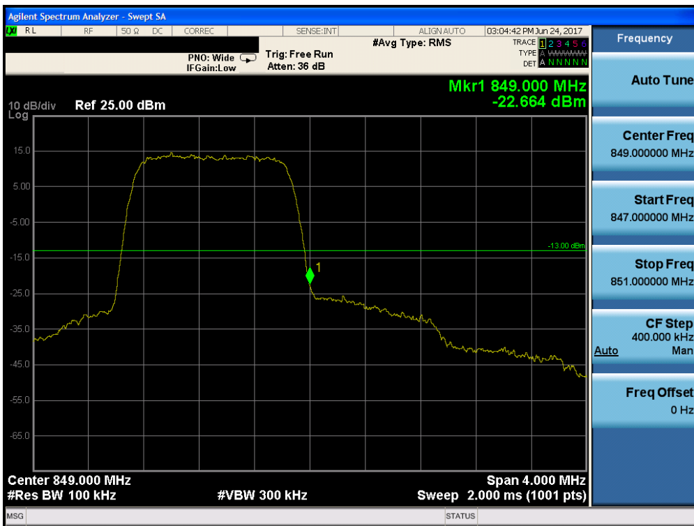
Plot 7-36. Upper Band Edge Plot (Band 5/26 – 1.4MHz QPSK – RB Size 6)
