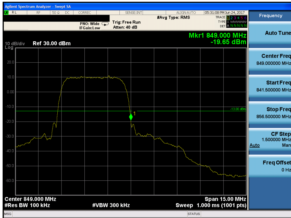
Plot 7-12. Band Edge Plot (Cellular WCDMA Mode – Ch. 4233)
