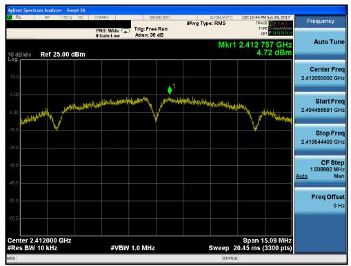
Plot 7-10. Power Spectral Density Plot (802.11b - Ch. 1)
