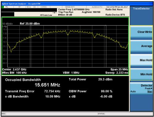
Plot 7-2. 6dB Bandwidth Plot (802.11b - Ch. 6)
