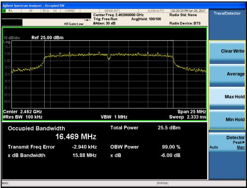
Plot 7-6. 6dB Bandwidth Plot (802.11g - Ch. 11)
