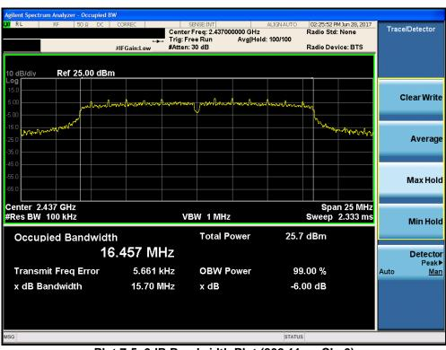
Plot 7-5. 6dB Bandwidth Plot (802.11g - Ch. 6)
