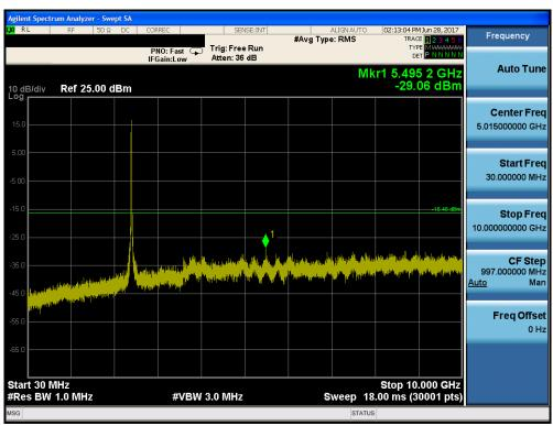
Plot 7-31. Conducted Spurious Plot (802.11b - Ch. 1)
