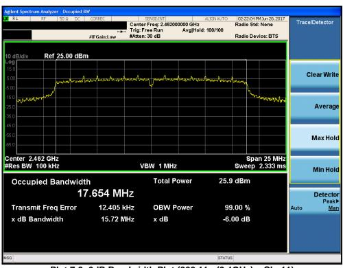
Plot 7-9. 6dB Bandwidth Plot (802.11n (2.4GHz) - Ch. 11)
