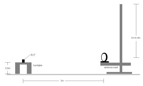
Figure 7-7. Radiated Test Setup < 30Mhz
