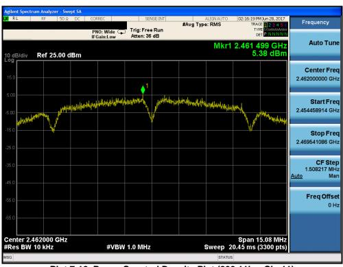
Plot 7-12. Power Spectral Density Plot (802.11b - Ch. 11)
