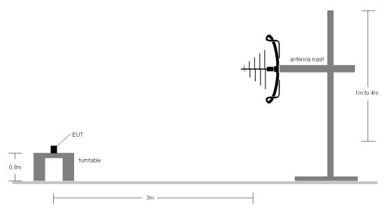
Figure 7-8. Radiated Test Setup < 1GHz
