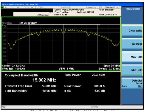
Plot 7-1. 6dB Bandwidth Plot (802.11b - Ch. 1)
