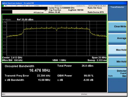
Plot 7-4. 6dB Bandwidth Plot (802.11g - Ch. 1)
