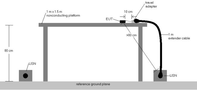
Figure 7-9. Test Instrument & Measurement Setup
