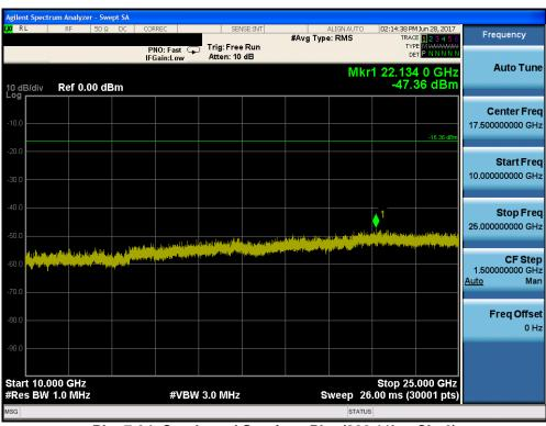
Plot 7-34. Conducted Spurious Plot (802.11b - Ch. 6)
