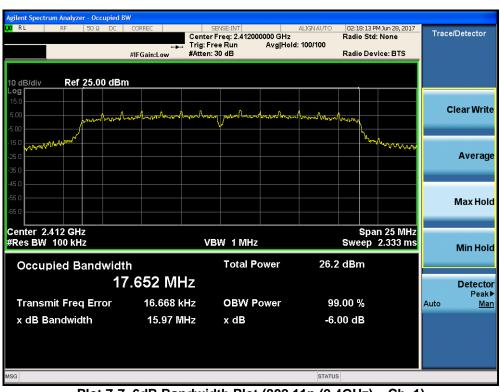
Plot 7-7. 6dB Bandwidth Plot (802.11n (2.4GHz) - Ch. 1)
