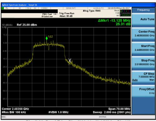
Plot 7-30. Band Edge Plot (802.11n (2.4GHz) - Ch. 13)
