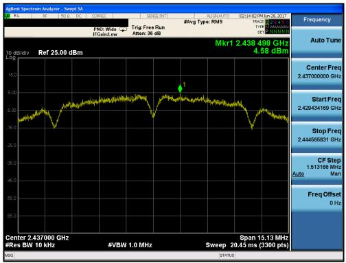
Plot 7-11. Power Spectral Density Plot (802.11b - Ch. 6)
