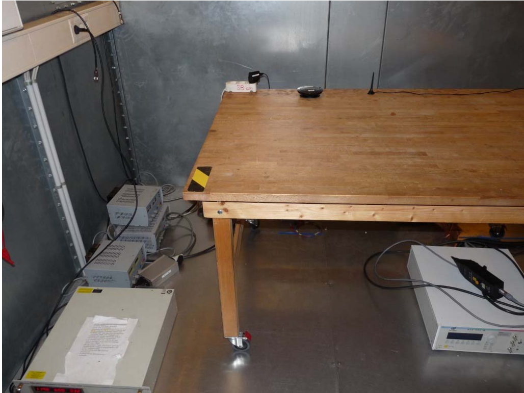
Photo 1: Test setup for conducted measurements (AC Port (power line)), unintentional transmission, EUT + AC/DC adapter
