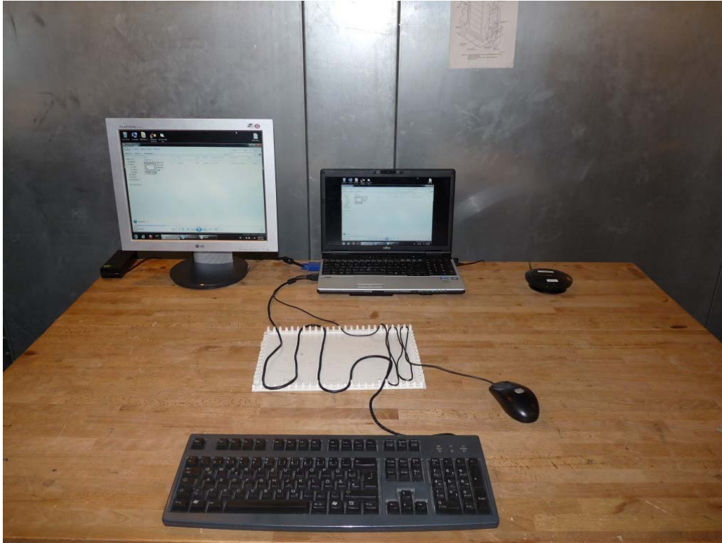
Photo 2: Test setup for conducted measurements (AC Port (power line)), unintentional transmission, EUT + computer peripheral setup
