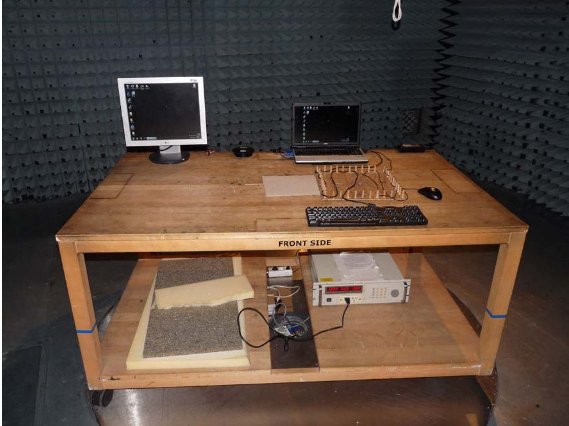
Photo 3: Test setup for radiated measurements (Enclosure, 30 MHz to 1 GHz), unintentional transmission, EUT + computer peripheral setup
