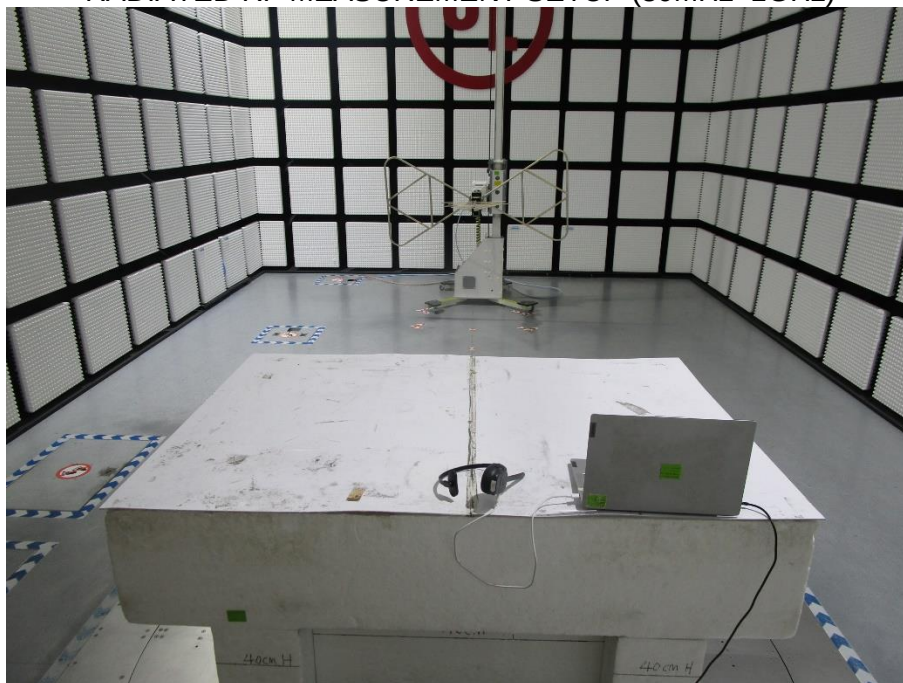
RADIATED RF MEASUREMENT SETUP (Below 30MHz)
