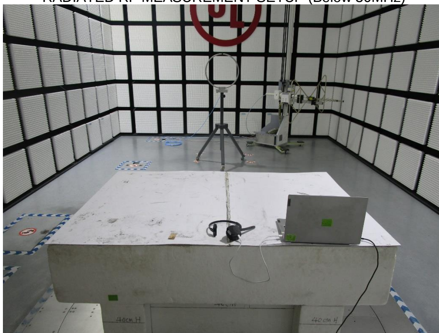
RADIATED RF MEASUREMENT SETUP (Below 30MHz)
