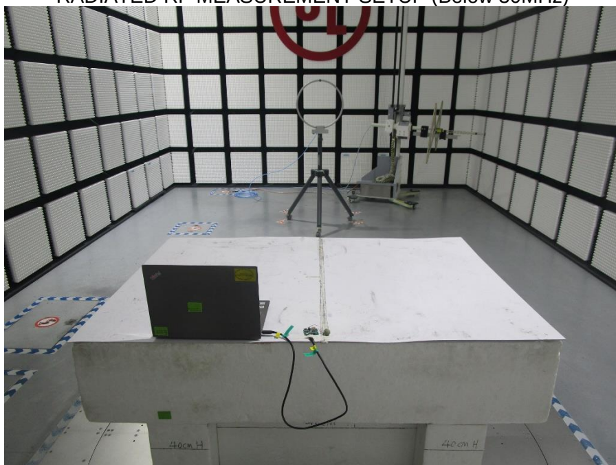
RADIATED RF MEASUREMENT SETUP (Below 30MHz)
