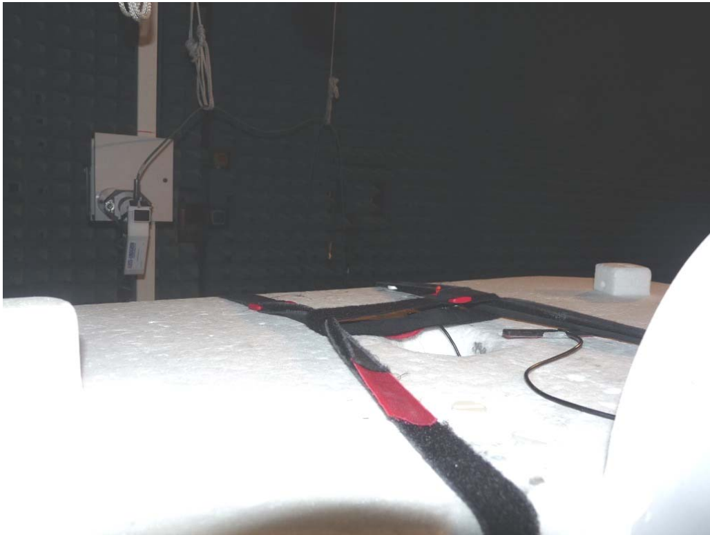
Photo 3: Test setup for radiated measurements (Enclosure, fully-anechoic chamber, 18-25 GHz, intentional radiator § 15)
