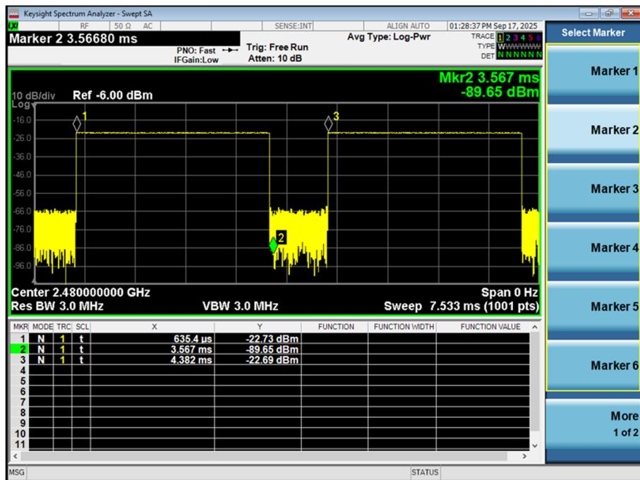
The SAR evaluation of this device selected BT-BR with the highest average power and the duty cycle is 78%
