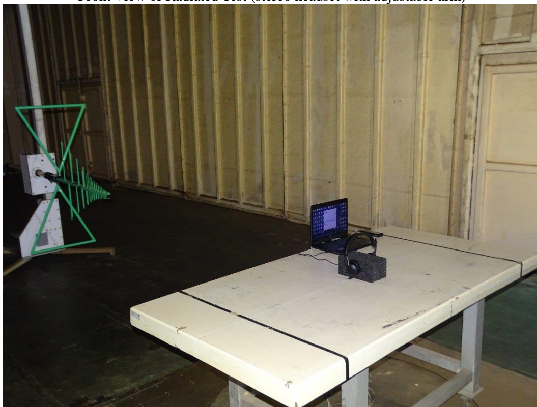
Back View of Radiated Test (stereo headset with adjustable arm)
