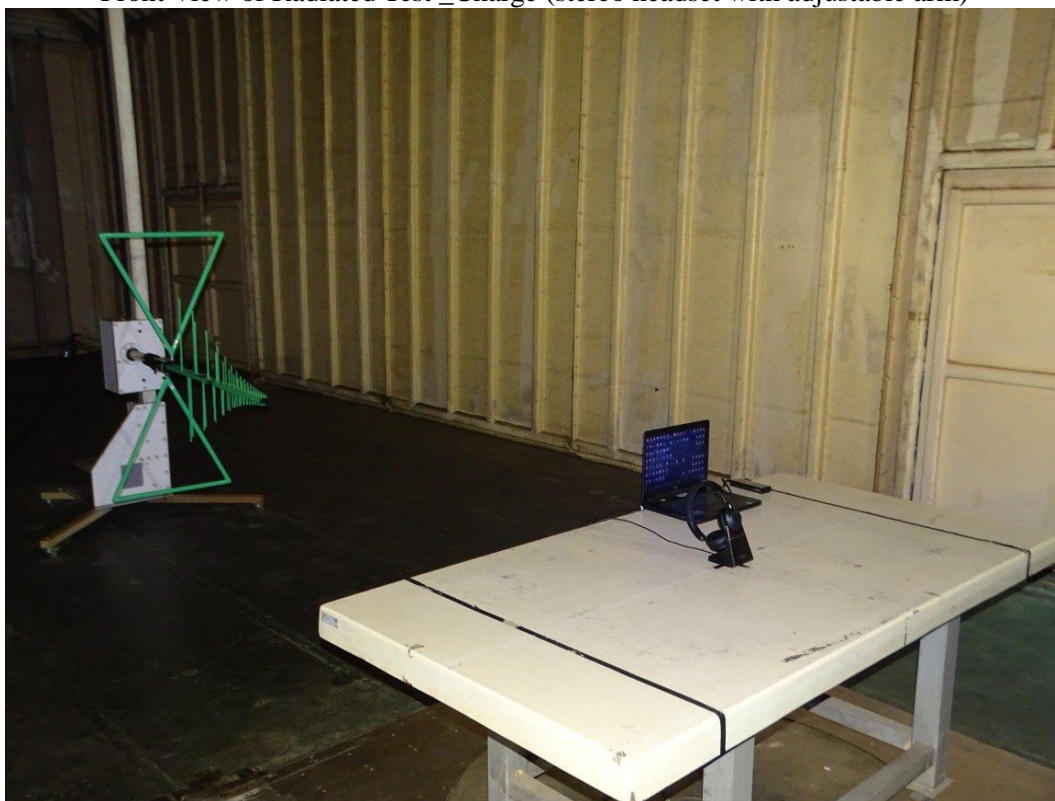
Back View of Radiated Test _Charge (stereo headset with adjustable arm)
