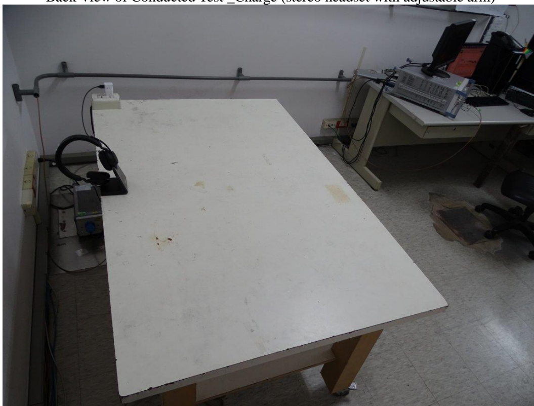
Back View of Conducted Test _Charge (stereo headset with adjustable arm)
