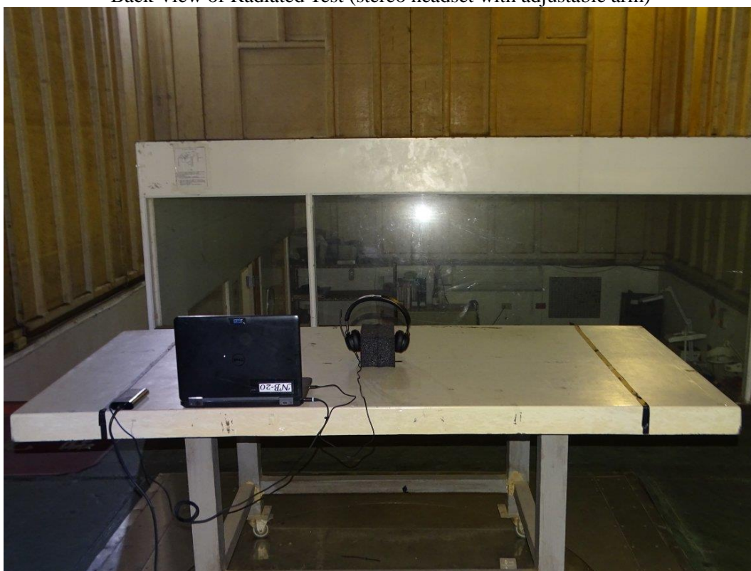
Back View of Radiated Test (stereo headset with adjustable arm)
