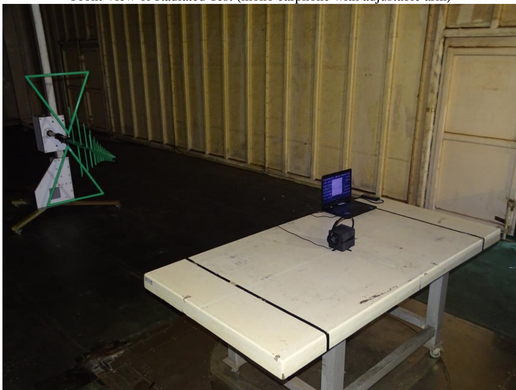
Back View of Radiated Test (mono earphone with adjustable arm)
