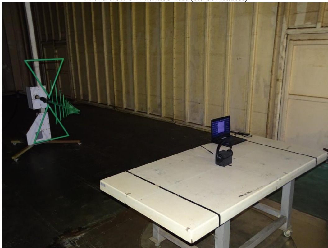
Back View of Radiated Test (stereo headset)
