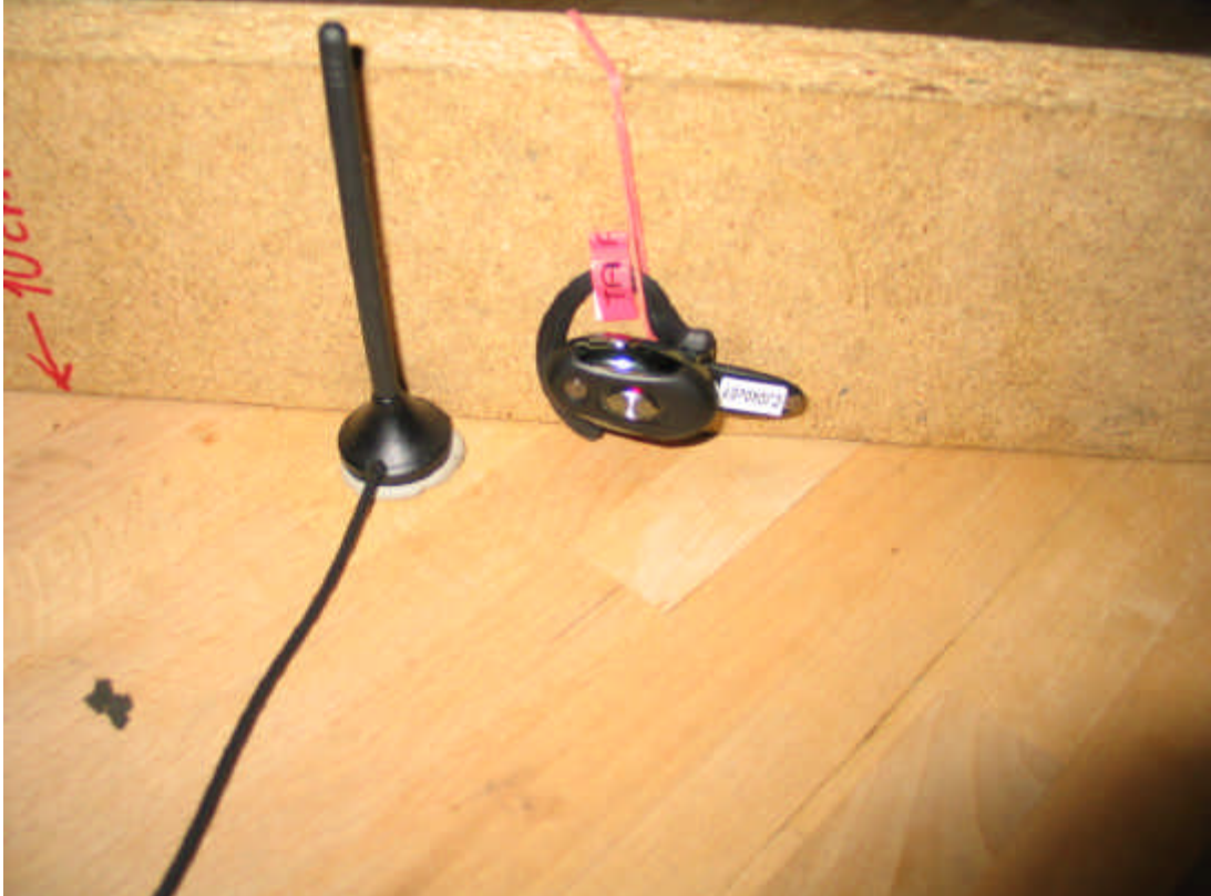
Photo 2: Test setup for radiated measurements (below 30 MHz, test on bottom side)
