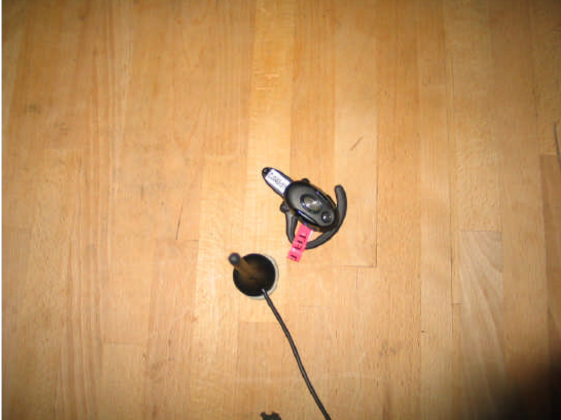
Photo 1: Test setup for radiated measurements (below 30 MHz, test on top side)
