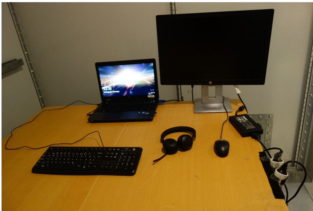
Test setup picture in Conducted Emission chamber
